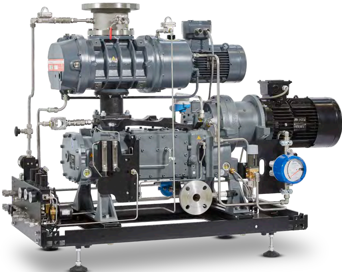
Figure 6.6: Combination of an EDS chemical dry screw pump (bottom) with an EH booster (top), typically used for freeze drying applications.
