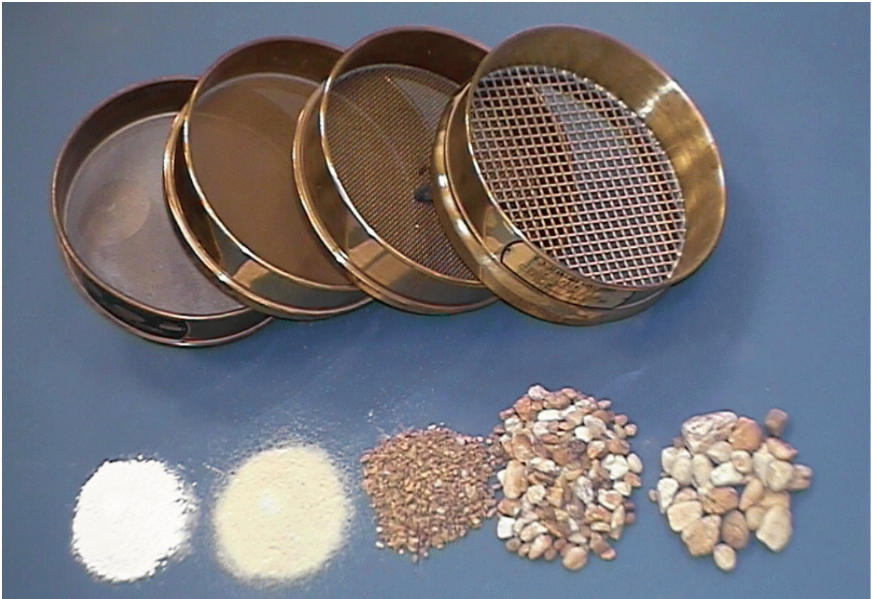
Figure 2. Example of laboratory sieves for mechanical analysis for grain size distributions. Shown (right to left) are sieve nos. 3/8-in (9.5-mm), No. 10 (2.0-mm), No. 40 (0.425 mm) and No. 200 (0.075 mm). Example soil particle sizes shown at the bottom of the photo include (right to left): medium gravel, fine gravel, medium-coarse sand, silt, and clay (kaolin) (FHWA, 2002b).
