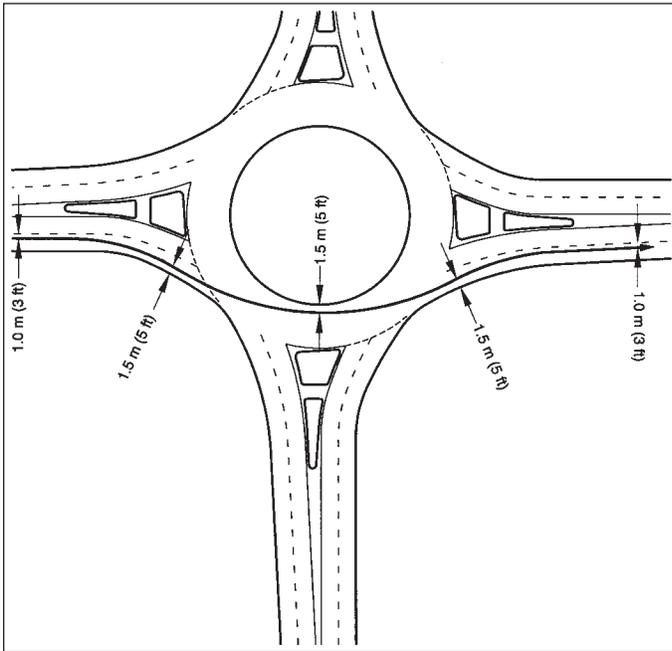
Exhibit 6-6. Fastest vehicle path through double-lane roundabout.
