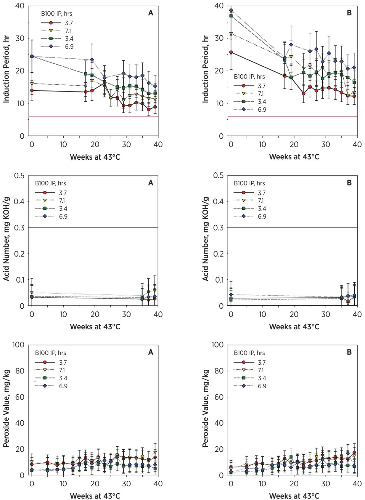
Figure 11. D4625 storage results for B5 blends made from B100 with varying levels of oxidation stability and two diesel fuels as measured by EN15751
