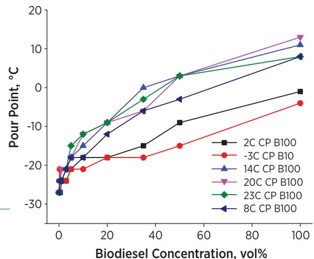
Figure 6 (top). Biodiesel/diesel blend cloud point test results
