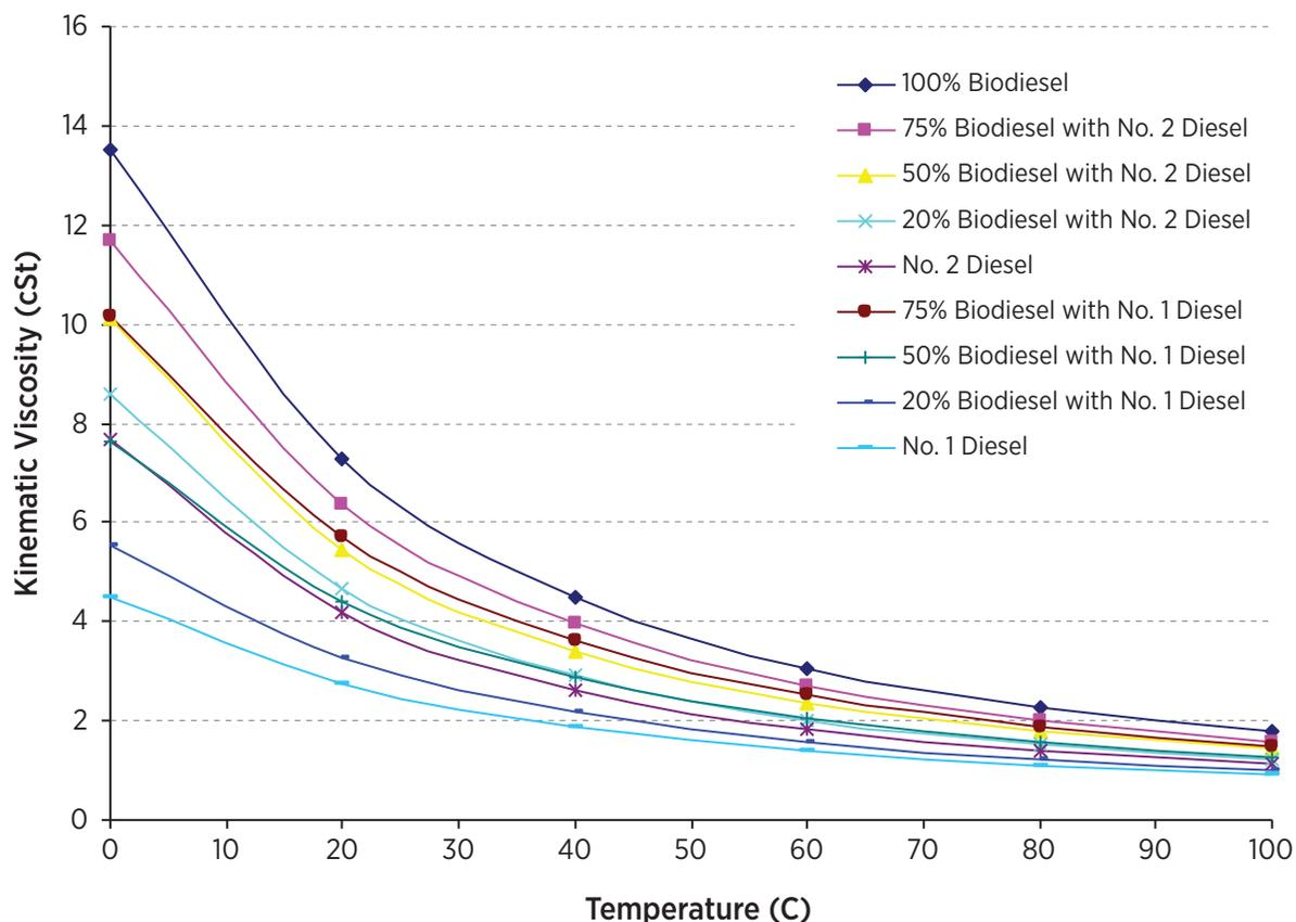
Figure 16. Kinematic viscosity for a commercial biodiesel in various blends<sup>30</sup>
