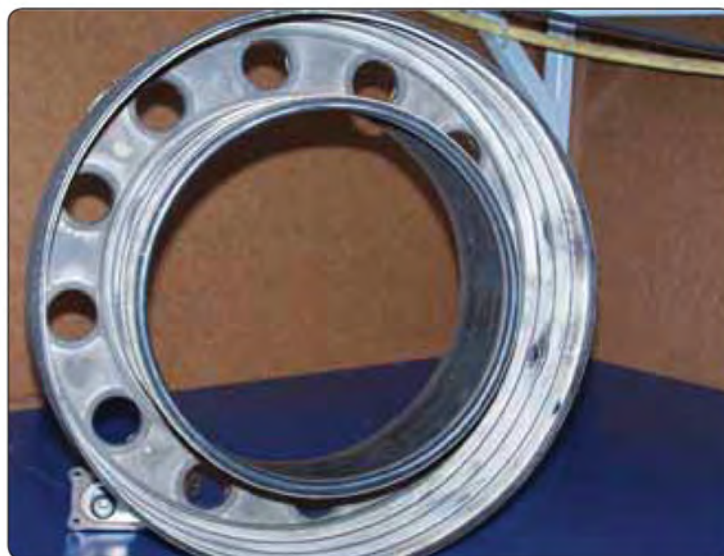
Figure 1-58. Annular combustion with chamber ceramic coating.
