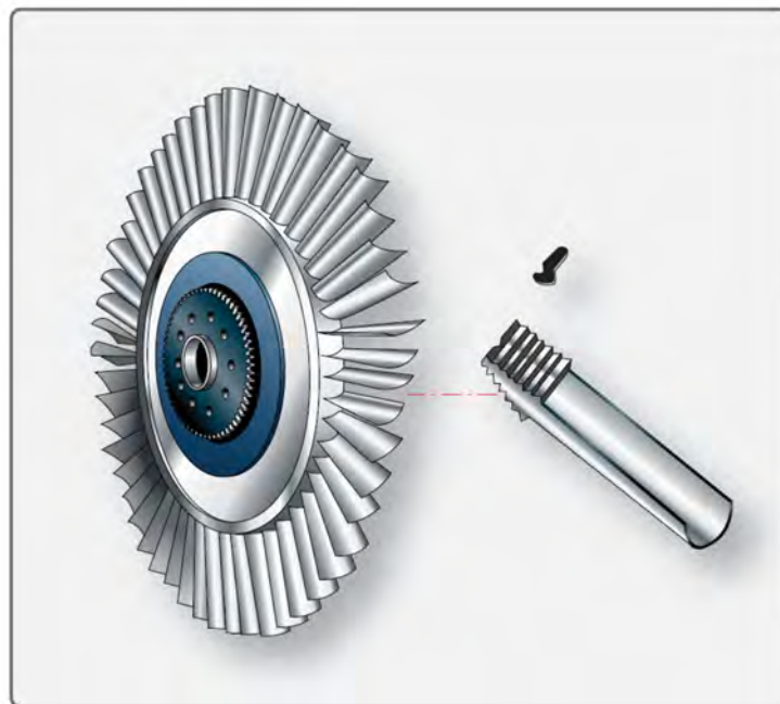
Figure 1-64. Turbine blade with fir-tree design and lock-tab method of blade retention.
