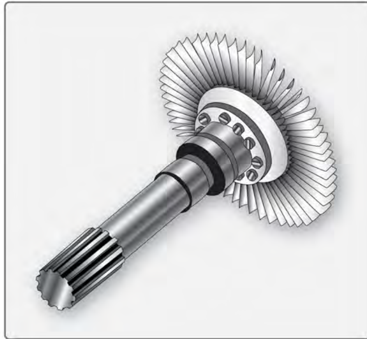
Figure 1-63. Rotor elements of the turbine assembly.
