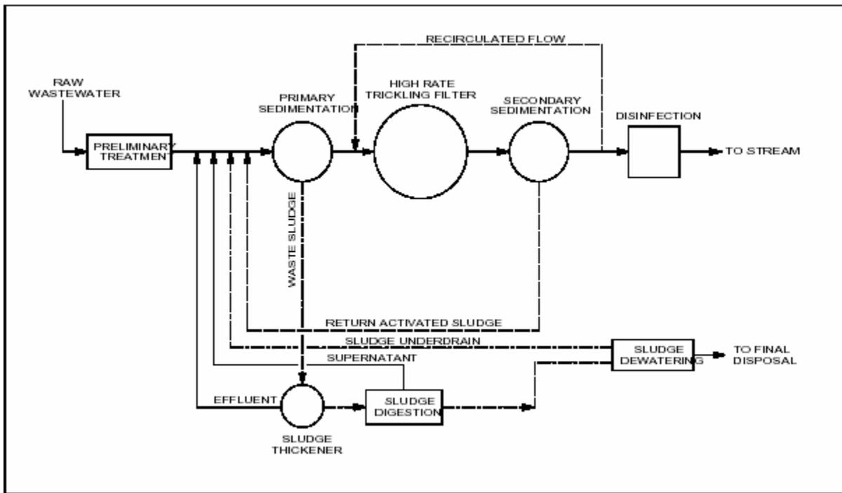
Figure 9-4 Sewage trickling Filter Process
