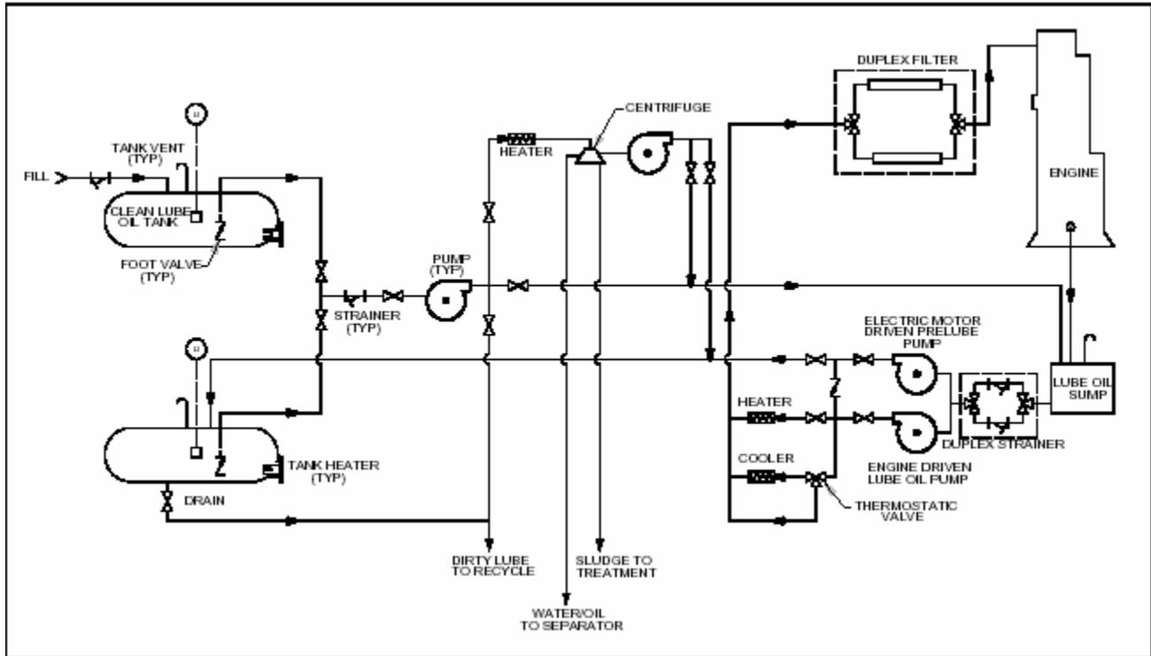
Figure 5-2 Schematic of a typical lube oil system
