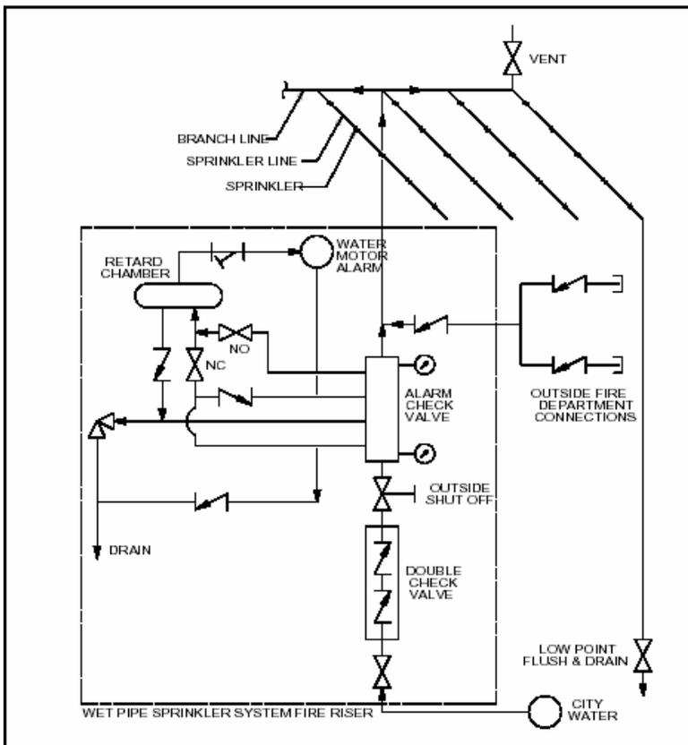
lines, fusible link sprinkler heads, vent and low point drain, tamper switches and post indicator valves.
