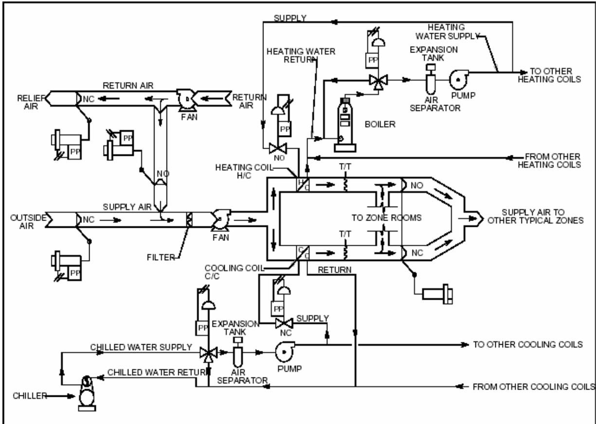
Figure 4-1. Schematic of a typical HVAC system
