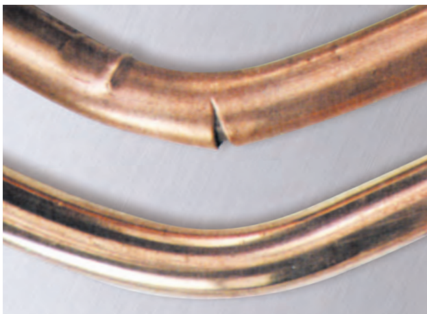
Figure 76. Copper bonded and copper clad earth rods.
