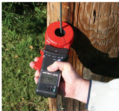
Figure 74. nVent ERICO test equipment for resistance and resistivity measurements.
