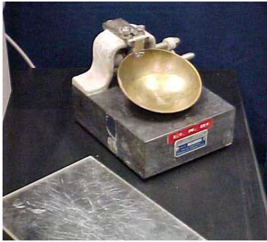
Figure 1-4. Some of the equipment used for Atterberg limits testing of soil.
