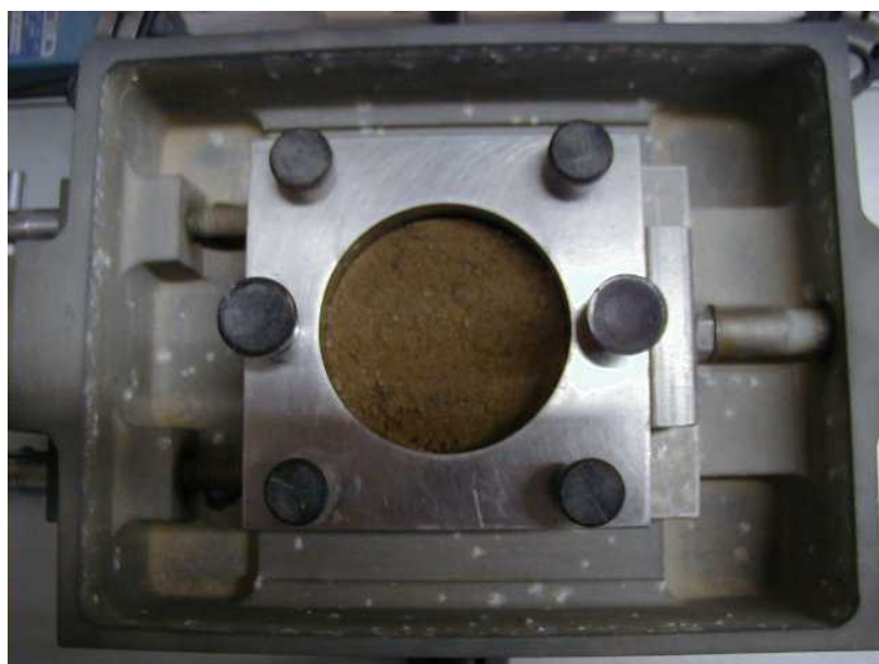
Figure 1-19. Soil sample mounted in direct shear testing apparatus (Photograph courtesy of GeoComp Corporation).
