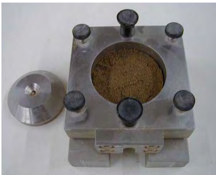
Figure 1-18. Direct shear testing box (Photograph courtesy of GeoComp Corporation).
