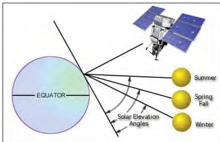
**Figure 1-13. Changes in sun elevation angle cause variations in the illumination conditions under which imagery is obtained.**
