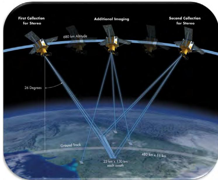
**Figure 1-12. Satellite agility enables the satellite to point in different directions and collect imagery off-nadir.**
