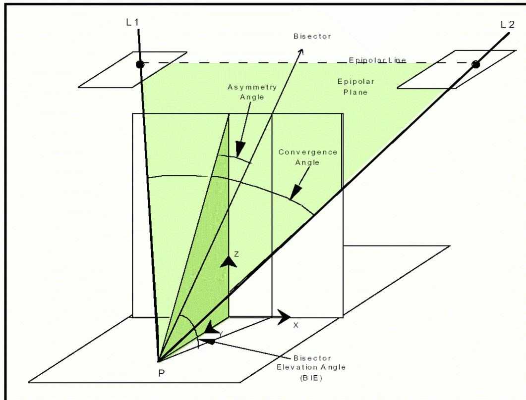
Figure 1-8. Epipolar plane, asymmetry angle, convergence angle, and bisector elevation angle (from STDI-0002)
