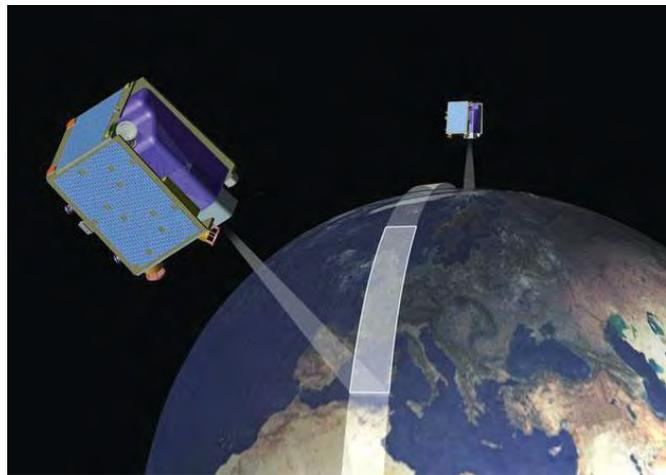
**Figure 1-16. RapidEye’s constellation approach permits a cumulative swath to be built up as multiple satellites view adjacent regions of the ground.**
