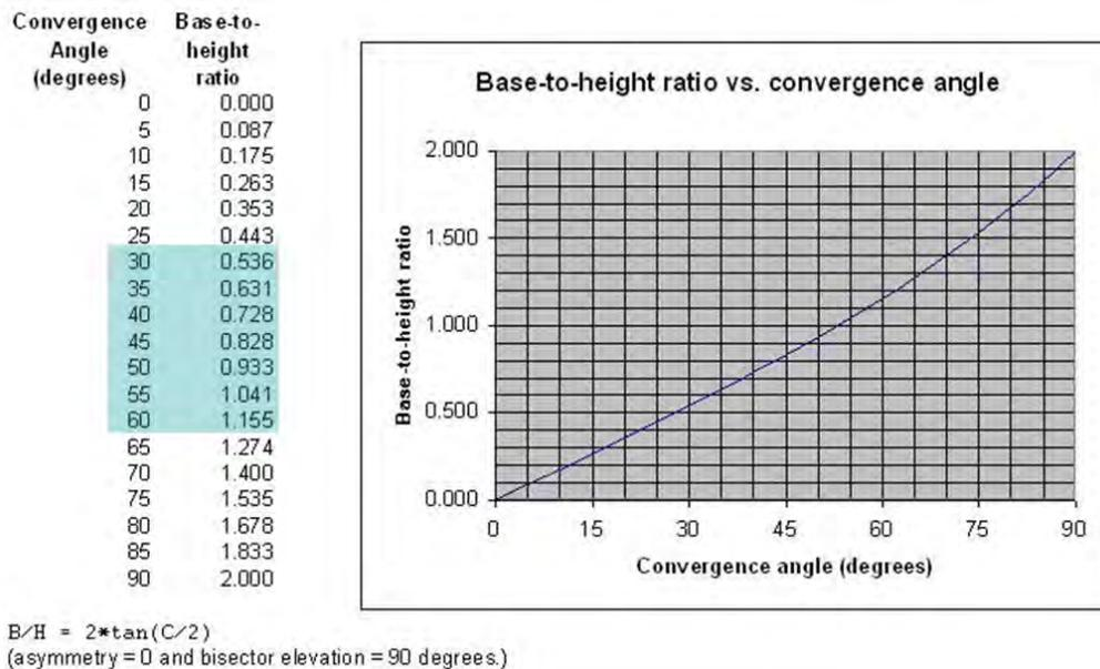
Figure 1-9. Relationship between stereo convergence angle and the base/height ratio.
