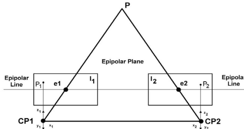
Figure 1-6. Epipolar Geometry
