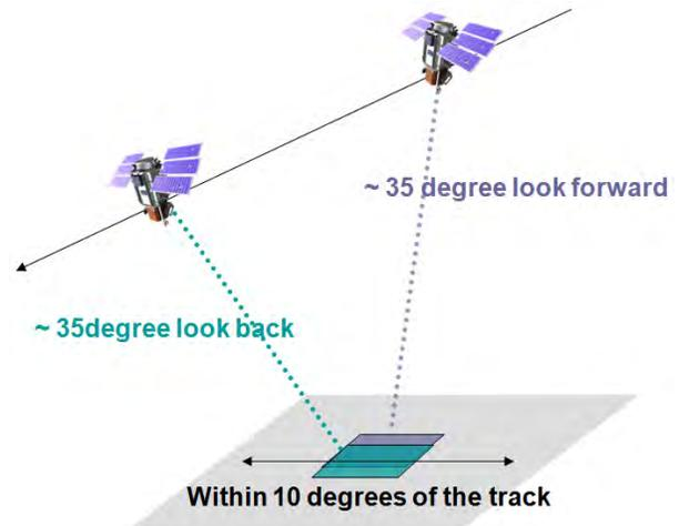
Figure 1-7. Satellite stereo image acquisition
