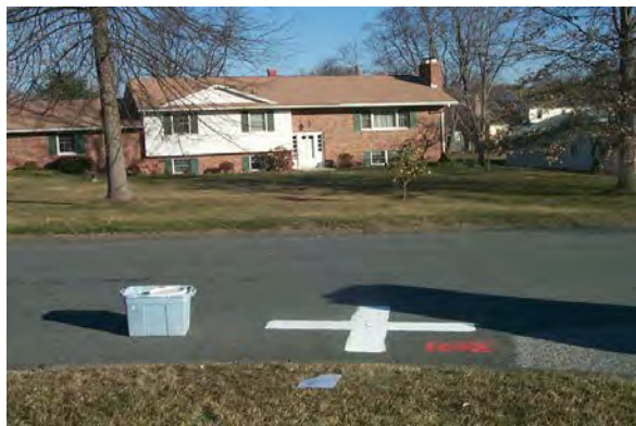
Figure 1-17. Painted photo control targets are commonly used when paved roads are available in desired locations.
