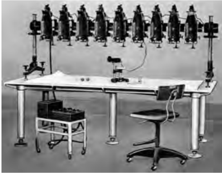
Figure 1-2. Multiplex projectors that physically replicate the geometry that existed when a flight line of nine aerial photos was taken. Without accurate relative orientation , the stereo images could never be focused in 3D in the stereo model, and without absolute orientation , the map would never fit ground control.
