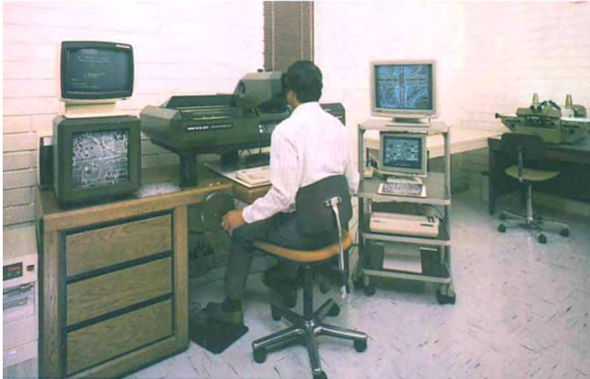
Figure 1-5. Wild BC2 analytical plotter that automates aerial triangulation and simplifies photogrammetric mapping processes. On the table to the right, a point marking and transfer device is shown that drills very small holes in the film emulsion for measurement of pass points and tie points used in aerial triangulation (AT).
