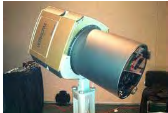
Figure 1-13. The UltraCam Eagle stores approximately 3.3 terabytes (3,800 images) per replaceable disk storage unit.
