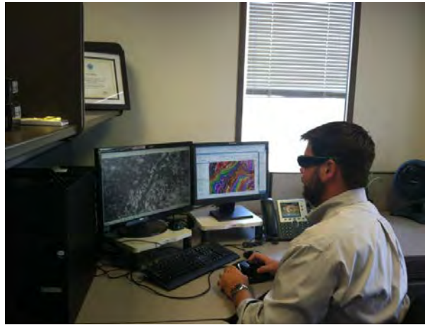
Figure 1-7. A digital stereo photogrammetric workstation running SOCET SET® photogrammetric software coupled with ArcGIS for real time display and analysis of data. This is used for softcopy photogrammetry and lidargrammetry.
