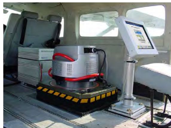
Figure 1-14. Leica ADS-40 Airborne Digital Sensor stores 480 GB in each of two mass memory units.
