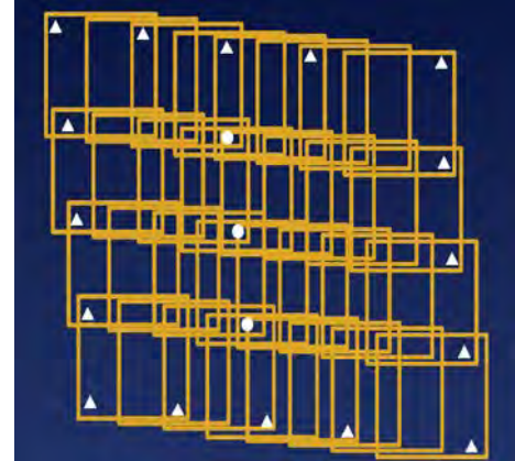
Figure 1-6. For an AT block adjustment, in addition to surveyed control points shown here, pass points and tie points are identified to “pass” X/Y/Z ground coordinates of points from one image to the next image in the same flight line and “tie” flight lines together.
