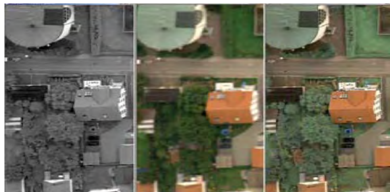
Figure 1-9. Higher-resolution panchromatic image and lower-resolution color image produced the “pan-sharpened” color image on the right.
