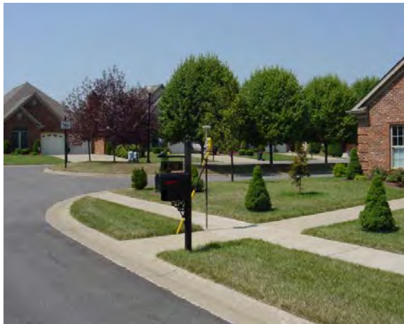
Figure 1-19. Photo control or QA/QC check point surveyed at 90° corner of grass and concrete.
