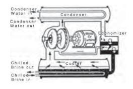
Figure 3-19: Free Cooling in Centrifugal Chillers
