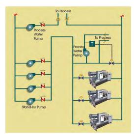
Figure 4-29: Auxiliary Condenser Water Loop
