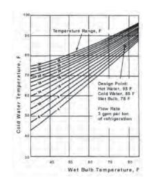
Cooling towers are relatively inexpensive when compared to the total cost of a chiller plant, and incremental increases in tower size and energy efficiency can be purchased at a very low cost. Skimping on the cooling tower is penny-wise and pound-foolish. Every effort should be made to optimize the selection of the tower. Matching larger fill volumes with lower fan capacities is a very good investment.
