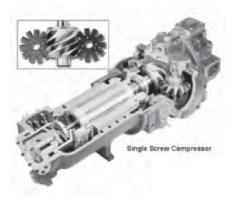
Figure 3-6: The Single Screw Compressor
