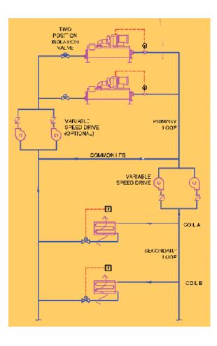
FIGURE 4-9: PRIMARY/SECONDARY VARIABLE FLOW PIPING, MULTIPLE CHILLERS, MULTIPLE COILS, MULTIPLE SERIES CHILLERS, MULTIPLE COILS
