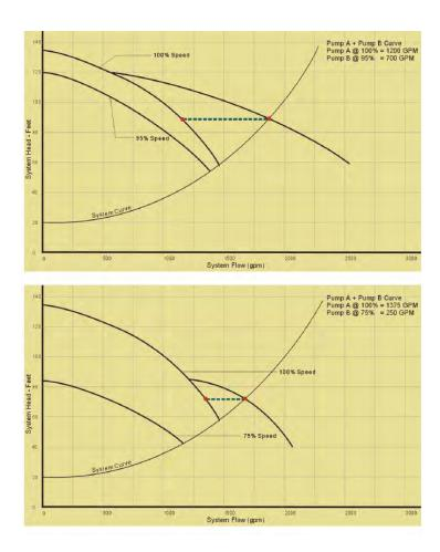
The system curve is accurate so long as nothing in the system changes. When two-way valves are incorporated into the system, the variable pressure drop created changes the system curve. This is important to understand because in a variable flow system with multiple two-way valves, there are many system curves that may represent the condition at various times.
