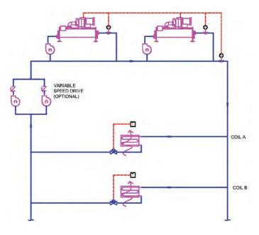
Another issue in primary/secondary piping is the size of the common piping (bypass pipe). In a multiple chiller system that is properly controlled, the maximum flow in the bypass should not exceed 110% to 115% of the flow from one chiller. However, in most cases the bypass line should be the same size as the supply and return header. There are two reasons for this:
