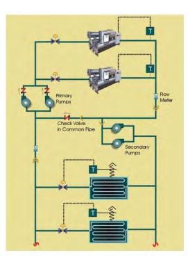
Figure 4-17: Check Valve in Common Pipe
