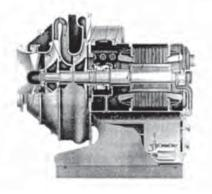
Figure 3-8: Hermetic Centrifugal Compressor
