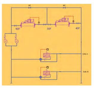
Figure 4-4: Constant-Flow System, Multiple Series Chillers, Multiple Coils
