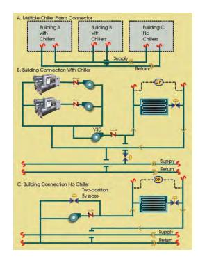
Figure 4-19: Connecting Multiple Chiller Plants on Secondary Side
