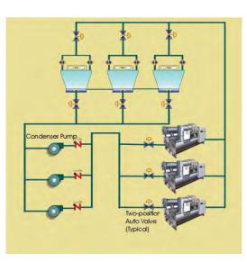
Figure 4-25: Headered Condenser Water Pumps Adding a standby pump (Figure 4-26) is very simple with this configuration. For large plants with more than three chillers, the number of condenser pumps can be reduced (for example, one pump for two chillers), as long as variable-speed drives are added to the pumps and valves are controlled to maintain a constant differential pressure at the chiller.
