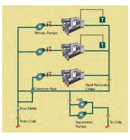
Figure 4-21 shows a configuration for a heat recovery machine that essentially puts the machine in series with the remaining chillers in the plant. Warm return water is pumped to the chiller then back into the return, thereby precooling the inlet water to the other chillers. The heat recovery machine can remove as much or as little heat as is needed for the heating load.
