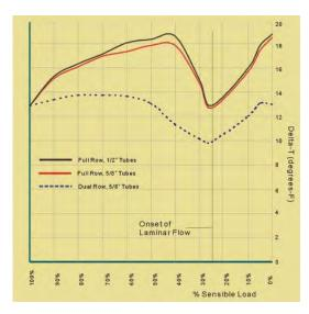
*Mitigation.* Designers specifying cooling coils should not only schedule the maximum performance of the coil but should also specify a "low load" coil condition so that coils are selected with low delta-T in mind. There are three ways to mitigate this problem:
