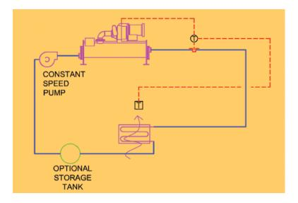
Figure 4-1: Constant-Flow System, Single Chiller, Single Coil
