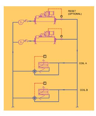
Figure 4-3: Constant-Flow System, Multiple Parallel Chillers, Multiple Coils
