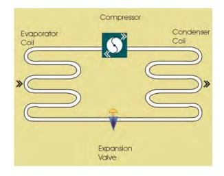
The refrigeration cycle diagram shows the relationship of these components, as does the pressureenthalpy chart, also known as a P-H diagram. These diagrams cover the liquid-vapor regions specific to the cycle refrigerant. The following is a description of the refrigeration cycle:
