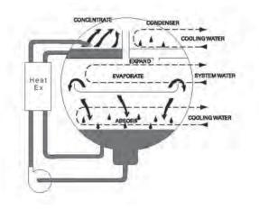
Figure 3-11: Absorption Refrigeration Cycle
