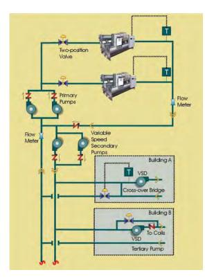
Figure 4-11: Primary/Secondary Variable Flow Piping, Tertiary Pumping
