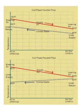
Figure4-16: Impact of Piping Coil Backwards
