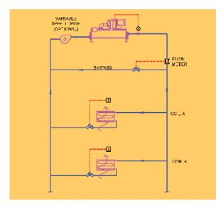
Figure 4-6: Primary-Only Variable Flow Piping, Single Chiller, Multiple Coils
