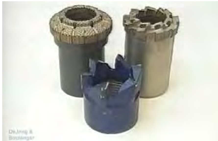
Figure 1-16. Coring bits: Diamond (top left), Carbide (top right), and Sawtooth (bottom center) (FHWA, 2002b).
