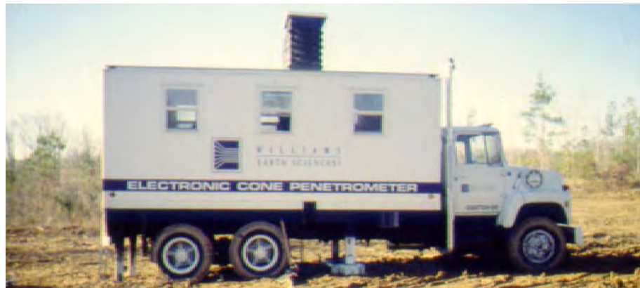
Figure 1-29. Cone penetration testing from cone truck.
