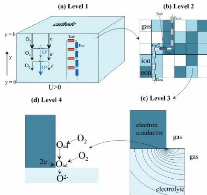
Figure 2-12 Overview of types of electrode models (9)
