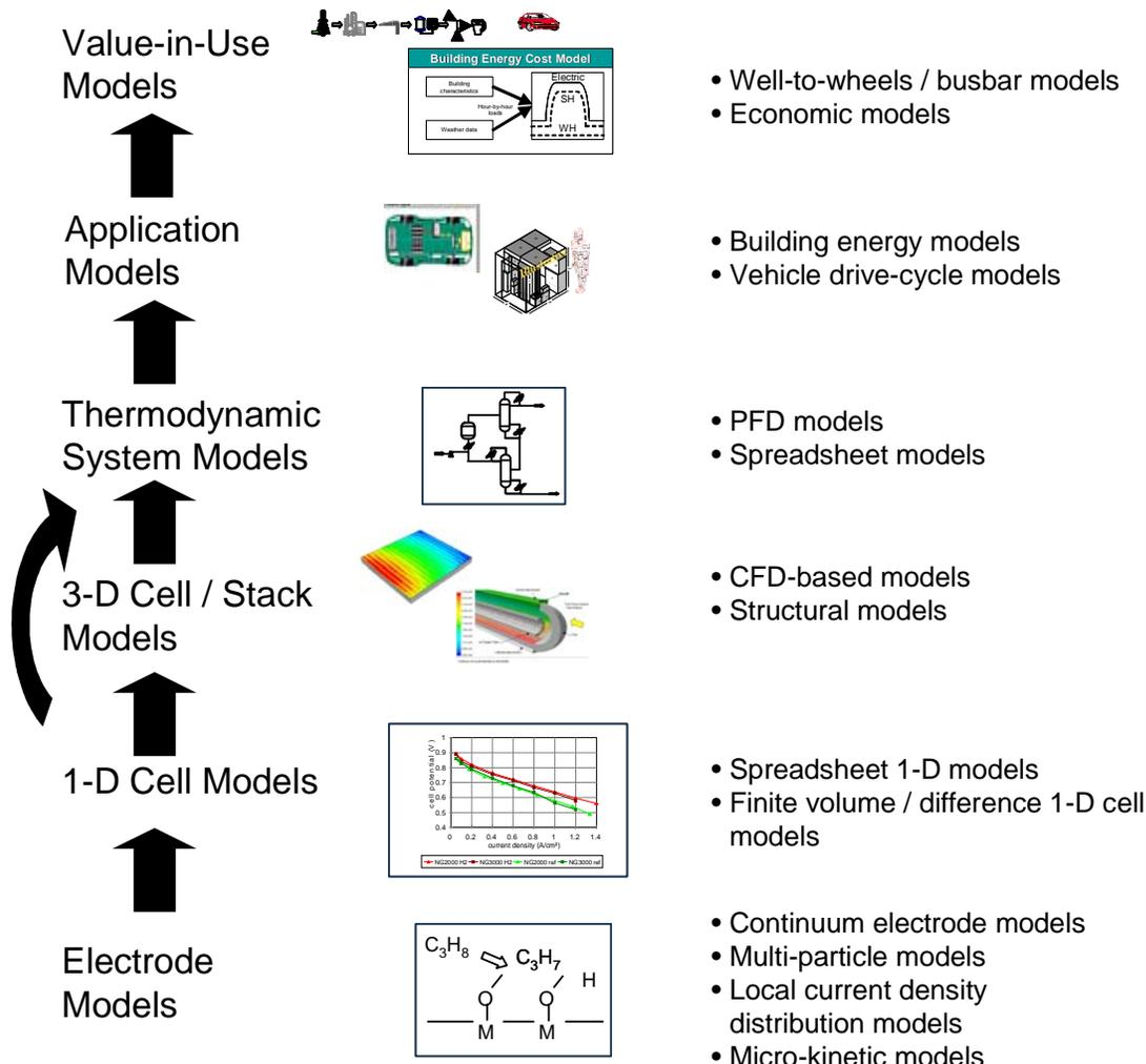
**Figure 2-9 Overview of Levels of Fuel Cell Models.**
