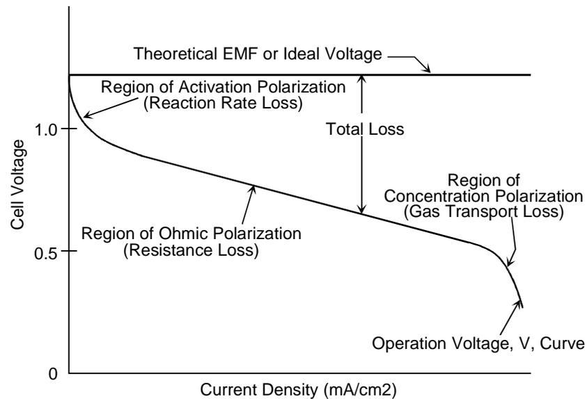
**Figure 2-3 Ideal and Actual Fuel Cell Voltage/Current Characteristic**
