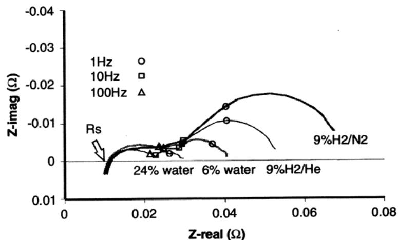
**Figure 2-5 Example of impedance spectrum of anode-supported SOFC operated at 850 °C (6).  $R_s$  is Ohmic resistance. Two measurements were with hydrogen/water vapor mixtures, and the other in diluted hydrogen.**
