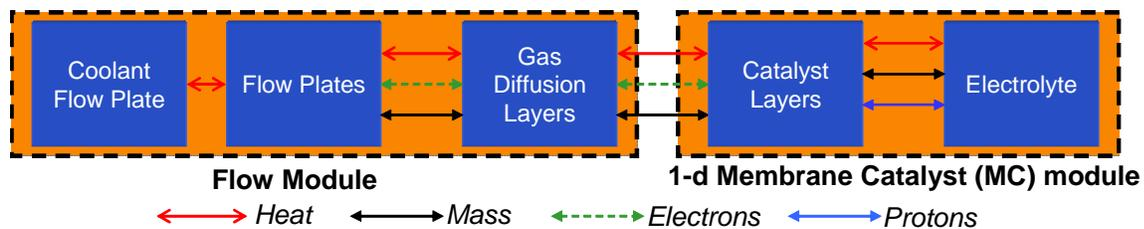
**Figure 2-11 Typical Phenomena Considered in a 1-D Model (17)**
