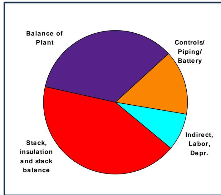
**Figure 1-14. Projected cost structure of a 5kWnet APU SOFC system. Gasoline fueled POX reformer, Fuel cell operating at 300mW/cm<sup>2</sup>, 0.7 V, 90 % fuel utilization, 500,000 units per year production volume.**
