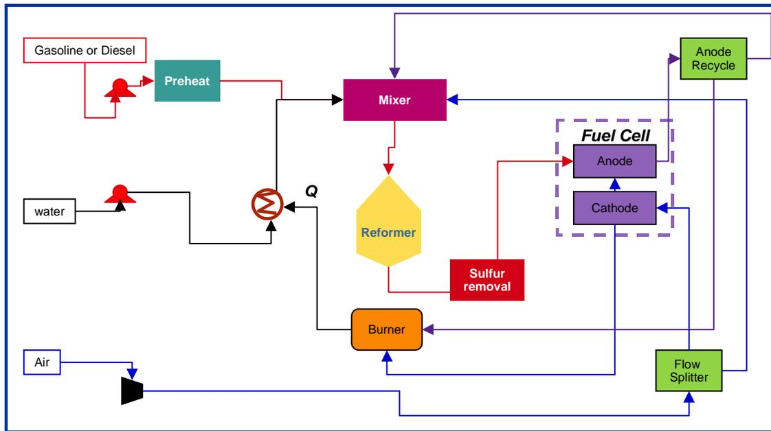
**Figure 1-12. Simplified process flow diagram of pre-reformer/SOFC system**
