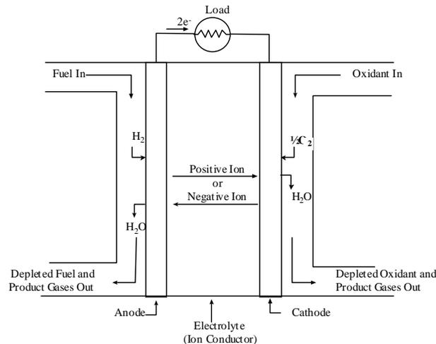
**Figure 1-1 Schematic of an Individual Fuel Cell**
