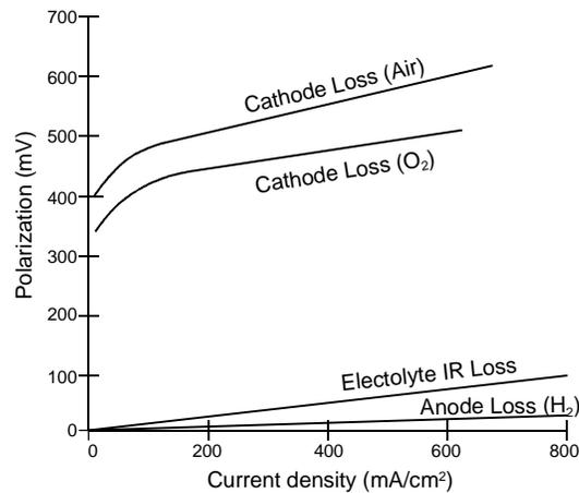
**Figure 2-6 Contribution to Polarization of Anode and Cathode**
