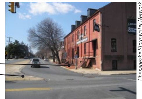
Figure 2-15. This simple road diet shows how two travel lanes are removed and replaced with one turn lane and two areas that could support green infrastructure practices.
