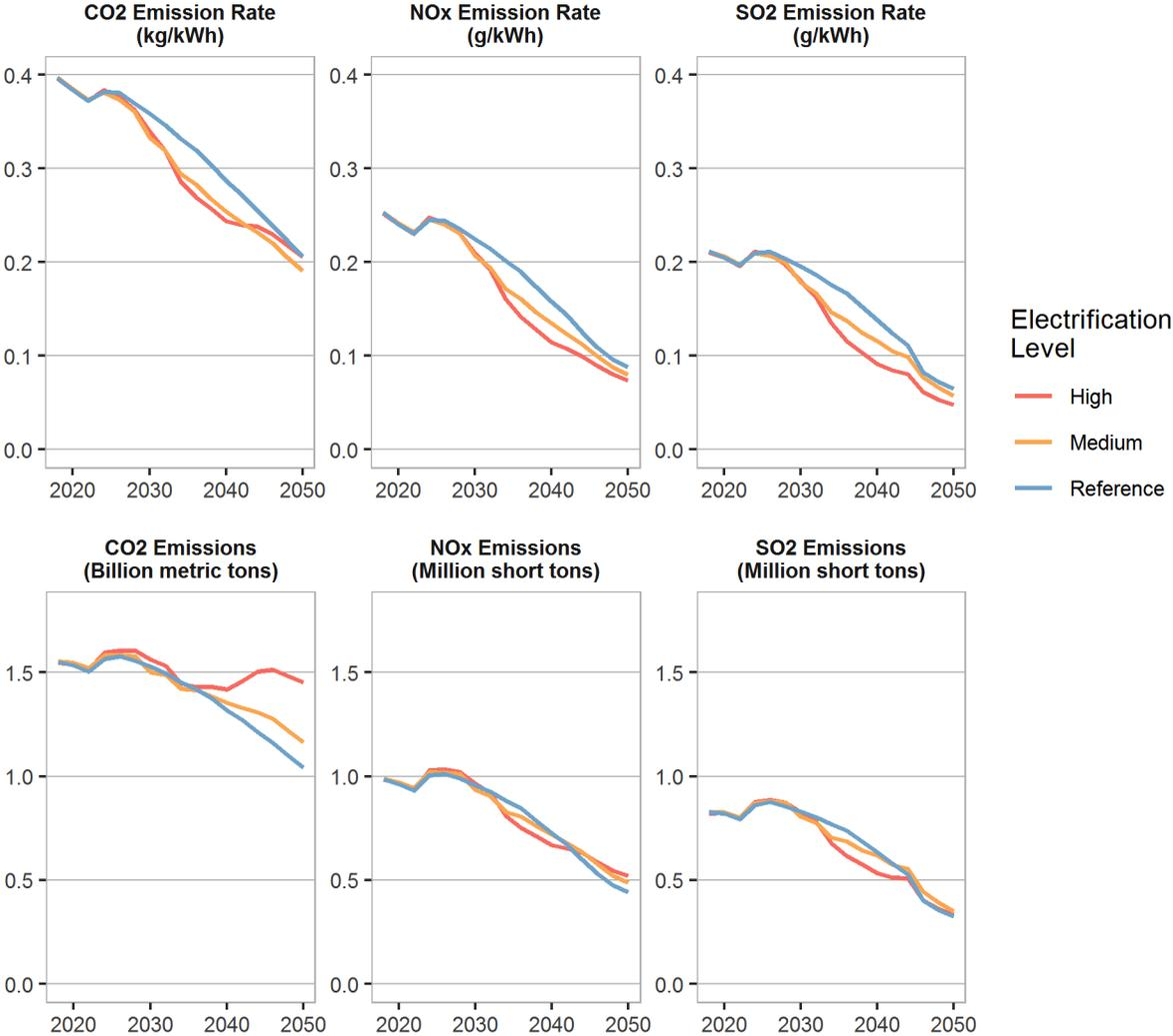
Figure 14. Electric sector emission rates (top) and absolute emissions (bottom) for CO<sub>2</sub> (left), NO<sub>x</sub> (middle), and SO<sub>2</sub> (right).
