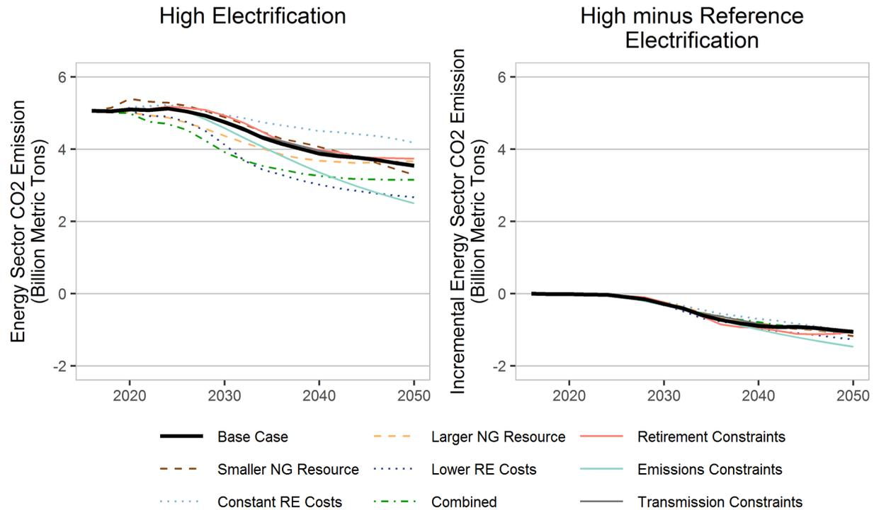
**Figure 27. Cumulative (left) and incremental (right) effects of High electrification on direct CO<sub>2</sub> emissions from the energy sector across all fuel, technology, and system constraint sensitivities**
