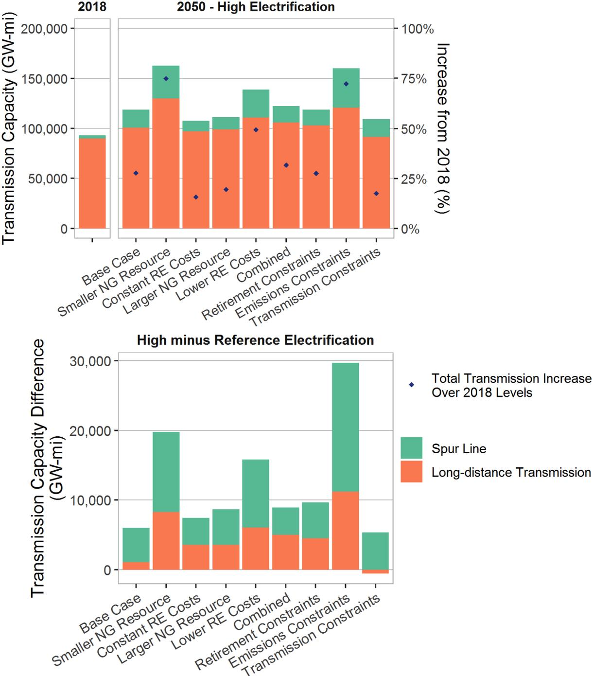
**Figure 22. Cumulative (top) and incremental (bottom) effects of High electrification on 2050 transmission capacity across all fuel, technology, and system constraint sensitivities**
