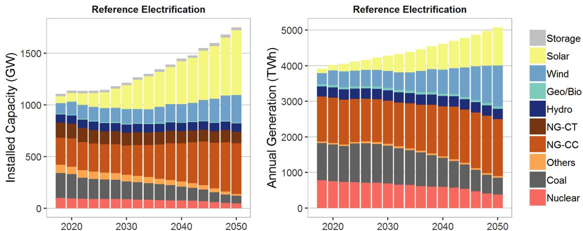
**Figure 4. Mixes of capacity (left) and generation (right) under the Base Case with Reference electrification and Moderate end-use technology advancement**
