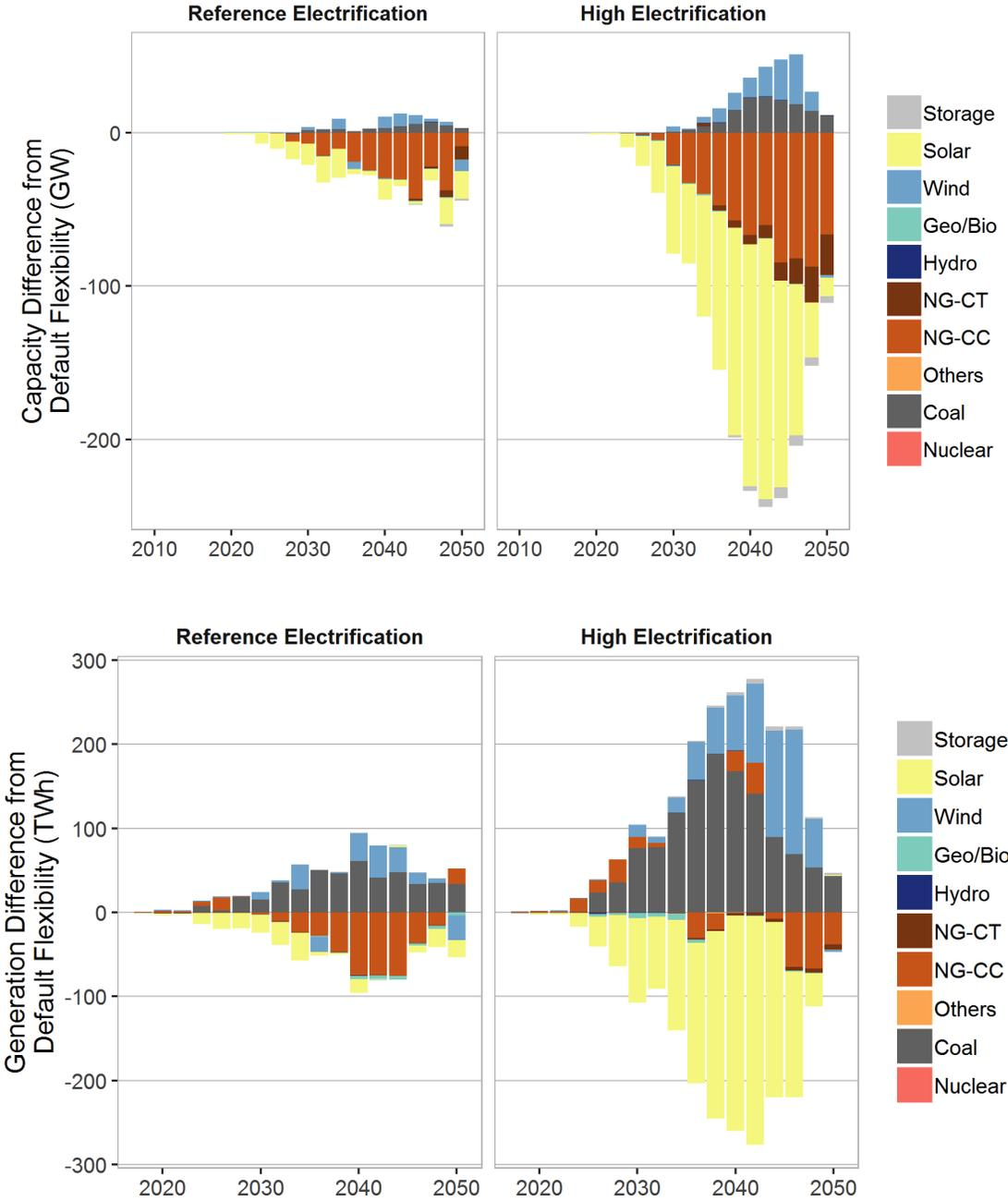
Figure 18. Effect of Enhanced demand-side flexibility (versus Base) on capacity (top) and generation (bottom) under Reference and High electrification
