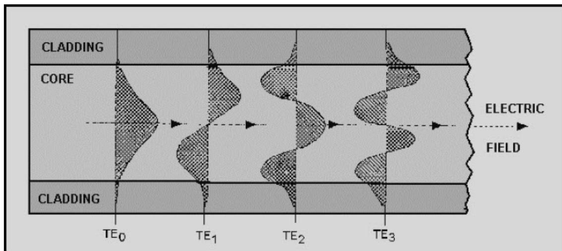
**Figure 2-18. - Transverse electric (TE) mode field patterns**
