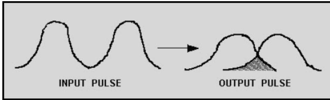
**Figure 2-17. - The spreading of a light pulse**
