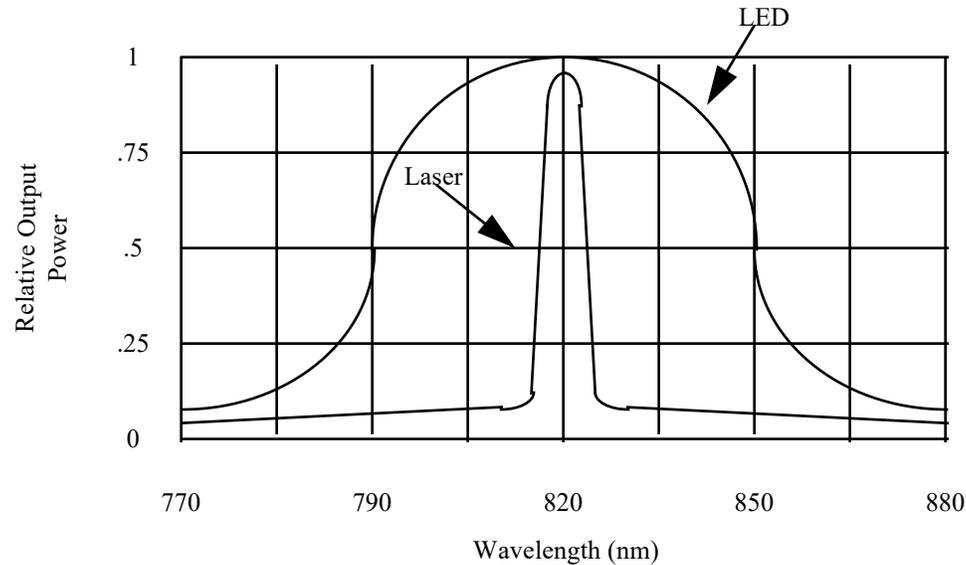
**Figure 1-4. - LED vs. Laser pulse width**
