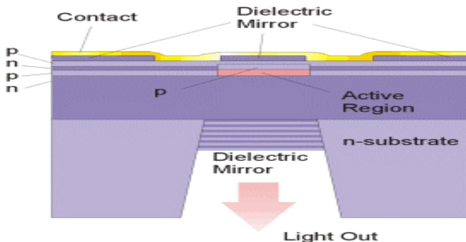
Figure 1-2. - Vertical Cavity Surface Emitting Laser
