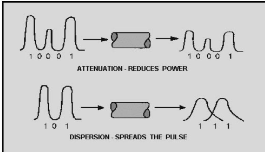
Figure 2-20. - Fiber transmission properties
