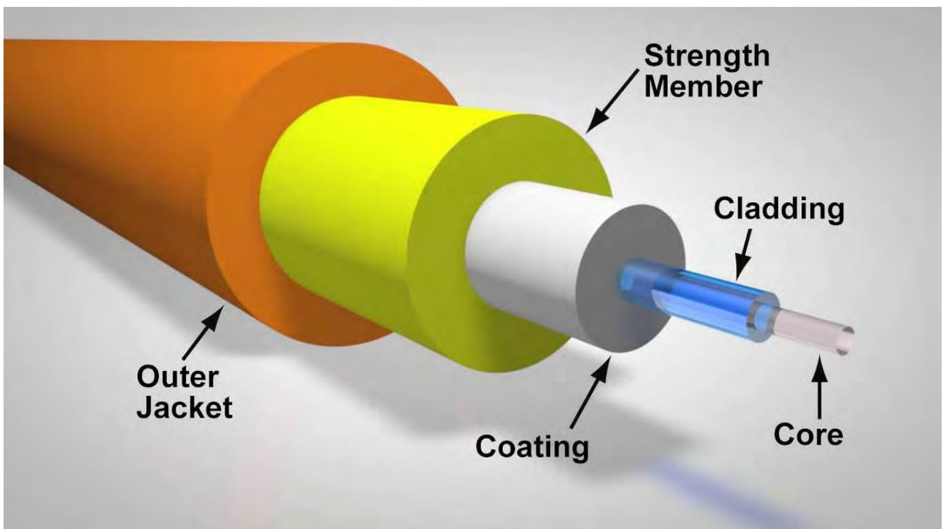
Figure 2-10. - Basic structure of an optical fiber
