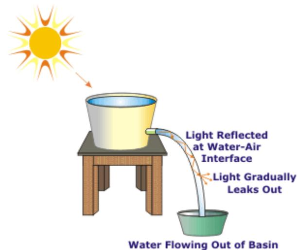
**Figure 1-7. - Early TIR (Total Internal Reflection) Demonstration**
