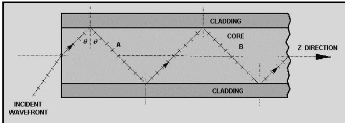
**Figure 2-16. - Wave front propagation along an optical fiber**
