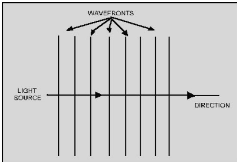
**Figure 2-15. - Plane-wave propagation**
