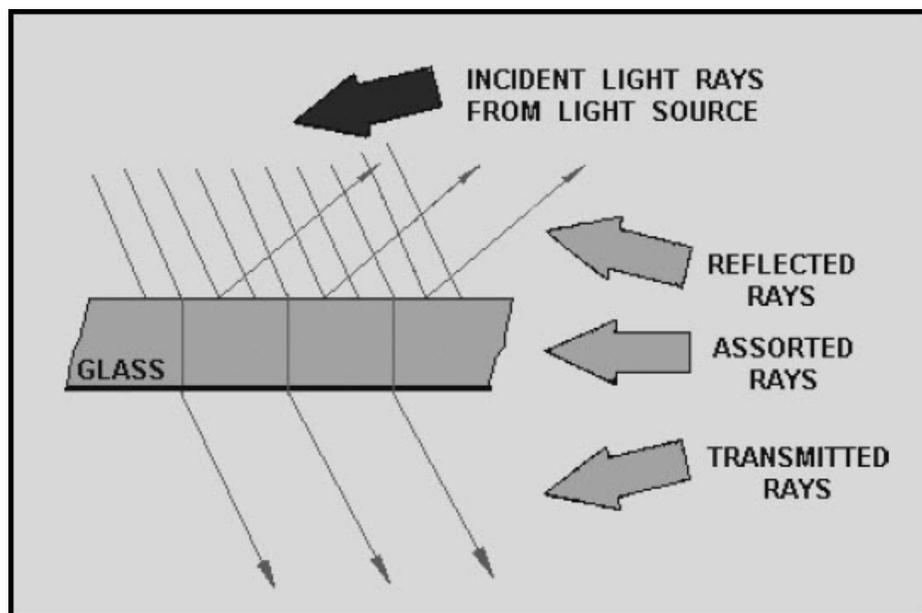
Figure 2-3. - Light waves reflected, absorbed, and transmitted
