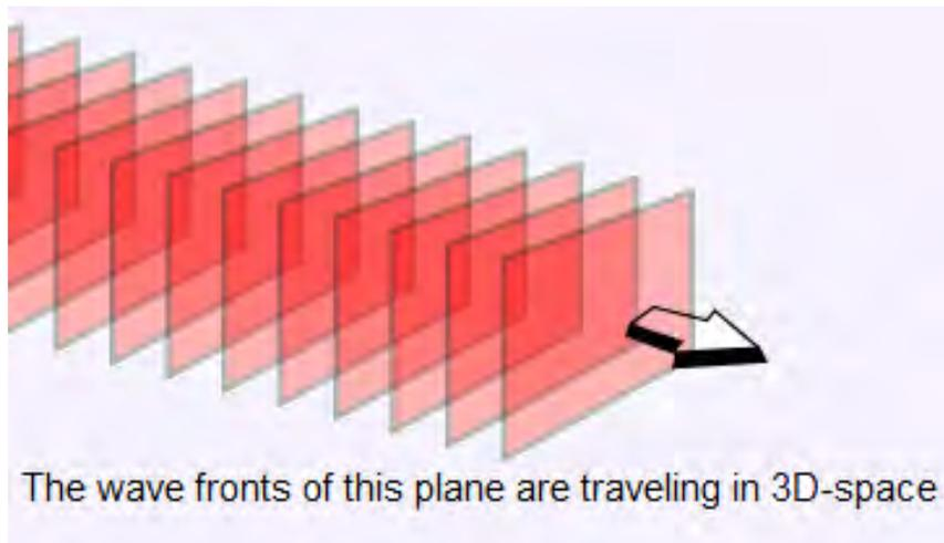
**PLANE WAVES.**—The mode theory suggests that a light wave can be represented as a plane wave. A plane wave is described by its direction, amplitude, and wavelength of propagation. A plane wave is a wave whose surfaces of constant phase are infinite parallel planes normal to the direction of propagation. The planes having the same phase are called the wave fronts. The wavelength ( $\lambda$ ) of the plane wave is given by:
