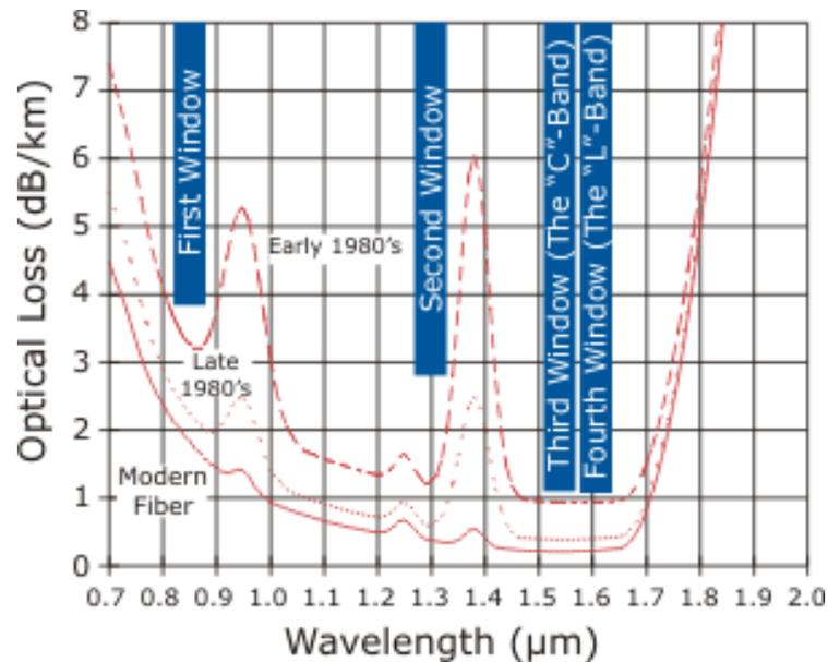
**Figure 1-8. - Four Wavelength Regions of Optical Fiber**
