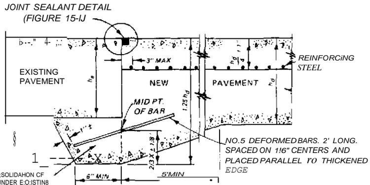
PLACEMENT AND CONSOLIDATION OF THE NEW CONCRETE UNDER EXISTING PAVEMENT SHOULD BE CARRIED OUT IMMEDIATELY PRIOR TO CONSTRUCTION OF THE NEW PAVEMENT. PLACEMENT OPERATIONS SHOULD BE TIMED SO THAT THE INITIAL CONCRETE IS STILL PLASTIC WHEN THE THICKENING OF THE CONCRETE PAVEMENT IS PLACED
