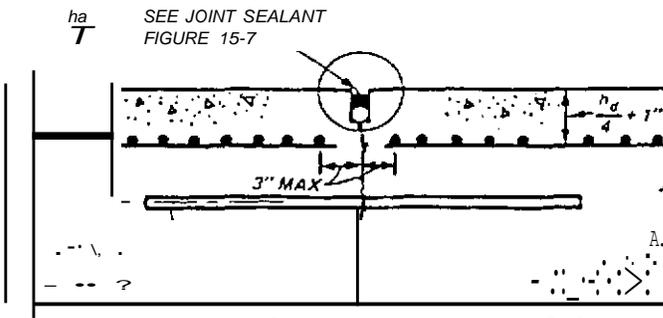
NO.5 DEFORMED STEEL TIE BARS 2'- 6" LONG AND SPACED 2'- 6" ON CENTERS
