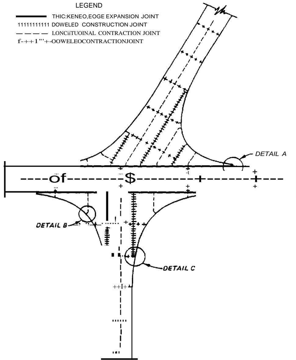
Figure 13-6. Typical Layout of Joints at the Intersection of Reinforced Rigid Pavement. (Sheet 1 of 2)
