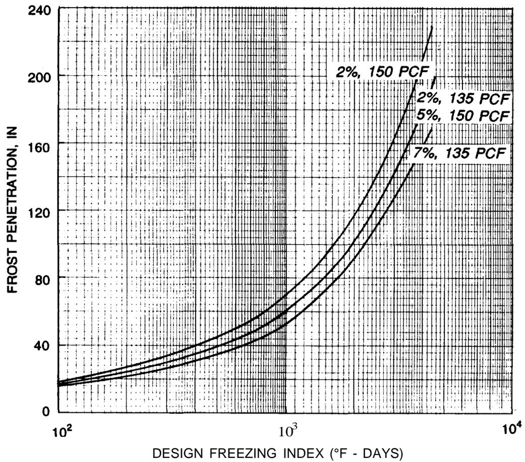
Figure 18-3. Frost Penetration Beneath Pavements. (Sheet 1 of 3)
