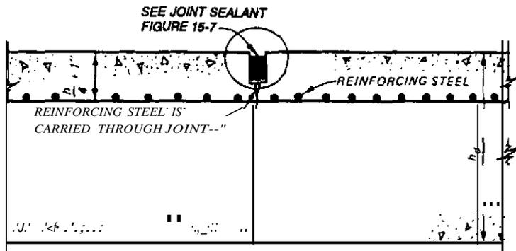
NOTE: SAW CUT WILL NOT EXTEND BELOW STEEL REINFORCING
