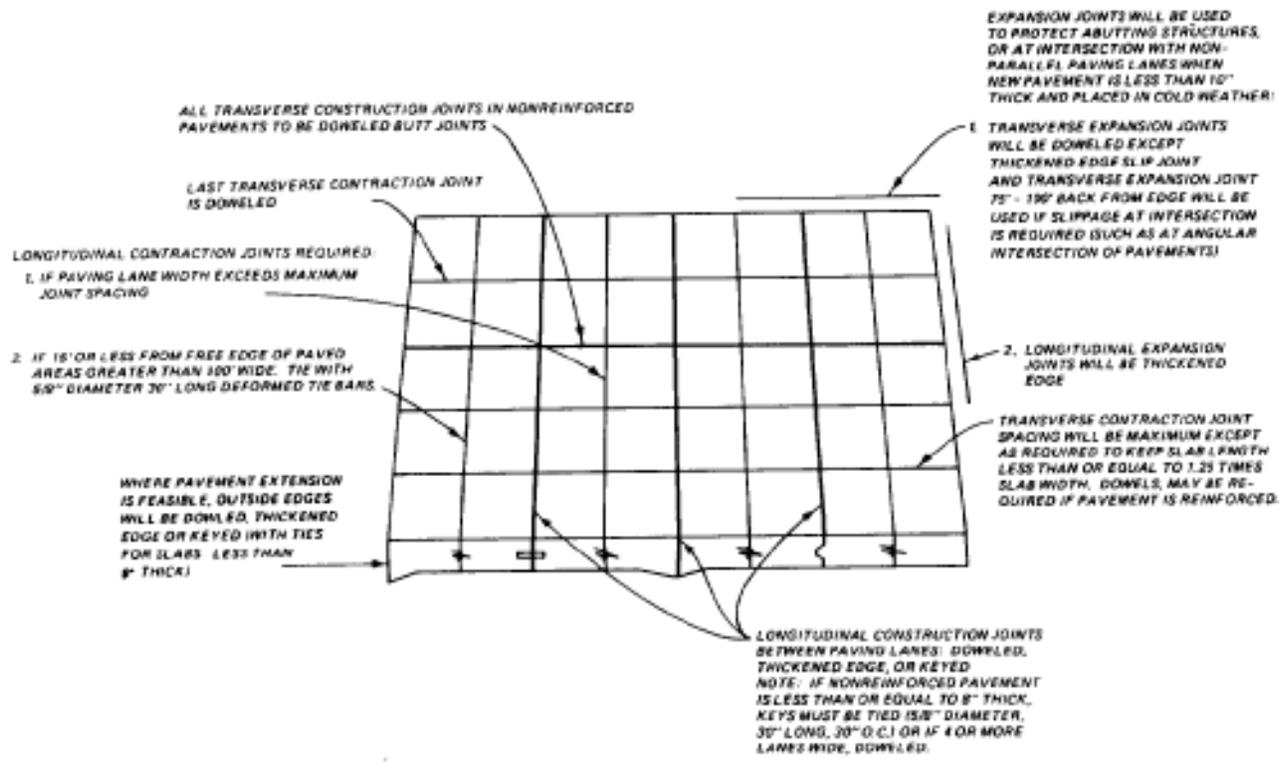
Figure 15-2. Joint Layout for Vehicular Parking Areas.
