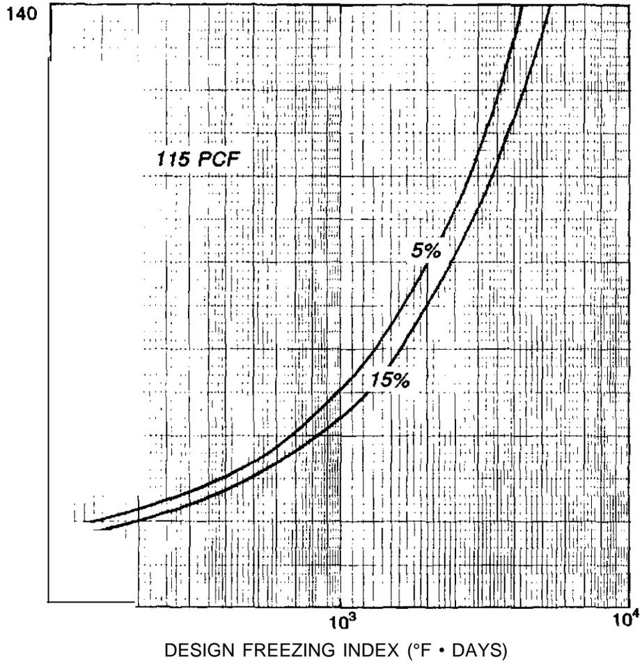
Figure 18-3. Frost Penetration Beneath Pavements. (Sheet 2 of 3)
