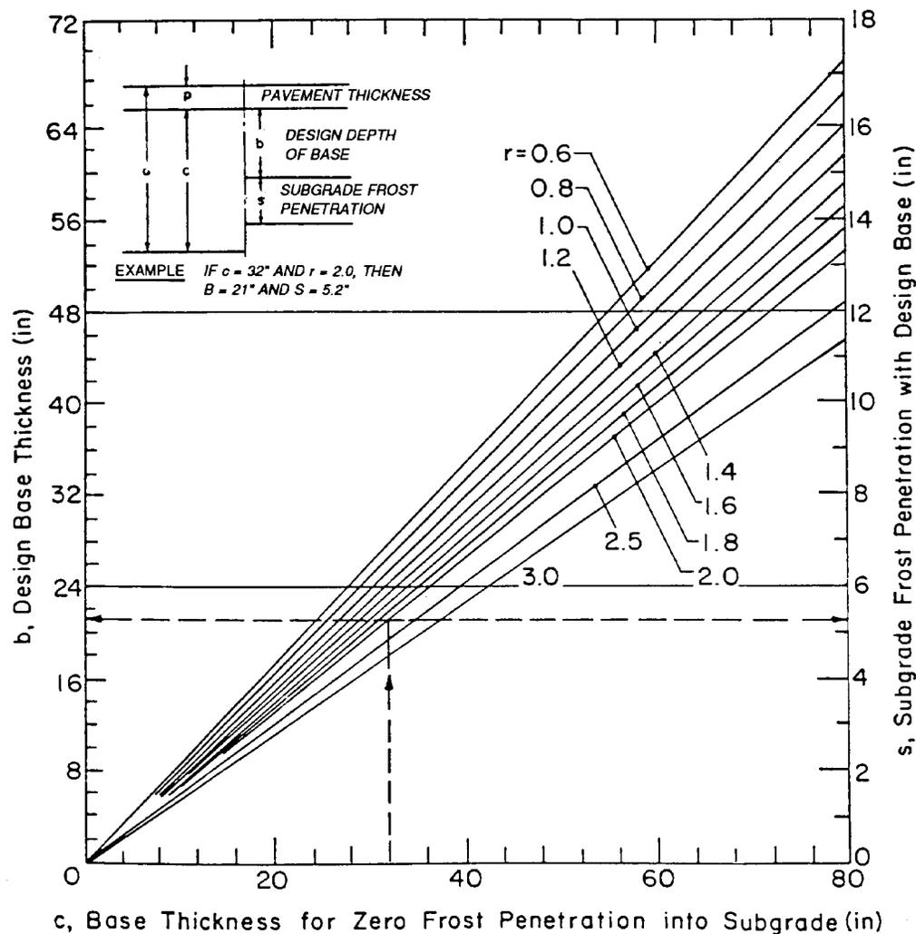
Figure 18-4. Design Depth of Nonfrost-Susceptible Base for Limited Subgrade Frost Penetration.
