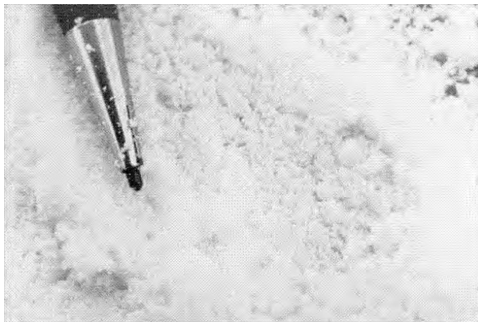
Figure 27. AN Prills after Temperature Cycling
