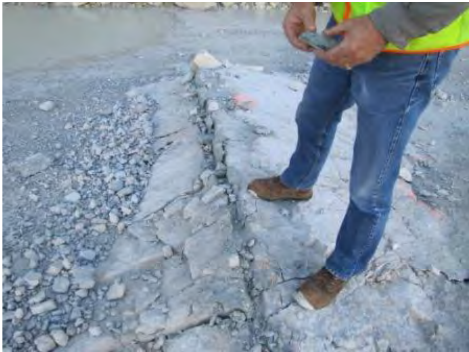
Figure 46. Heave in Quarry Floor Due to Unloading of the Rock by Blasting and Excavation.
