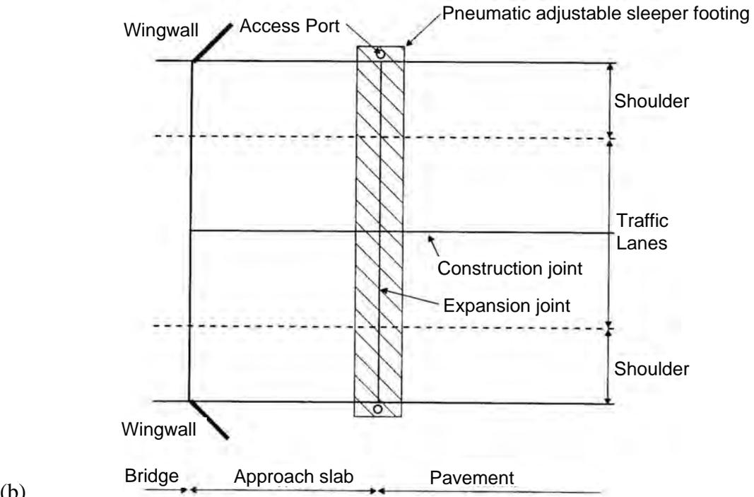
Note: This plan detail is only one way of handling the bridge/fill interface. An approach slab with expansion between the superstructure and the approach slab without a sleeper slab is another.
