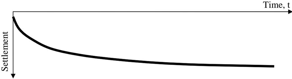
**Figure 1-14. Typical settlement-time curve for clay under an embankment loading.**
