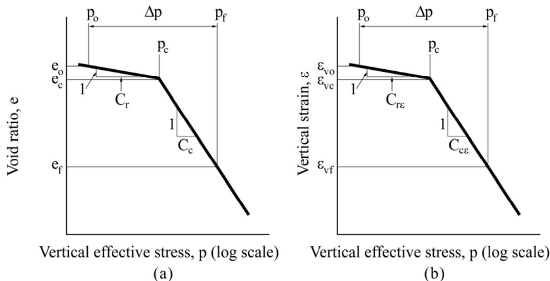
**Figure 1-11. Typical consolidation curve for overconsolidated soil, (a) Void ratio versus vertical effective stress and (b) Vertical strain versus vertical effective stress.**
