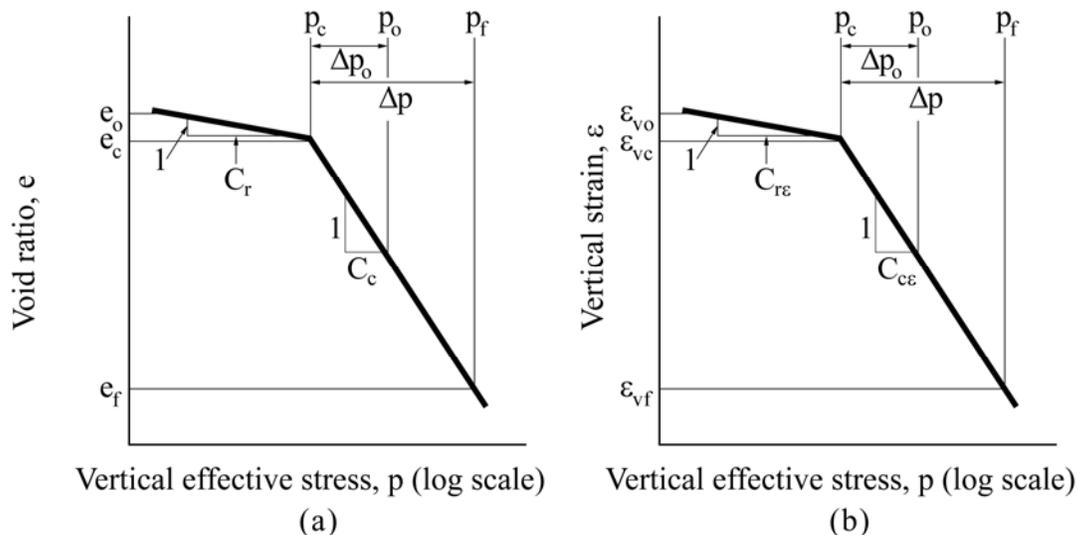
**Figure 1-12. Typical consolidation curve for under-consolidated soil – (a) Void ratio versus vertical effective stress and (b) Vertical strain versus vertical effective stress.**
