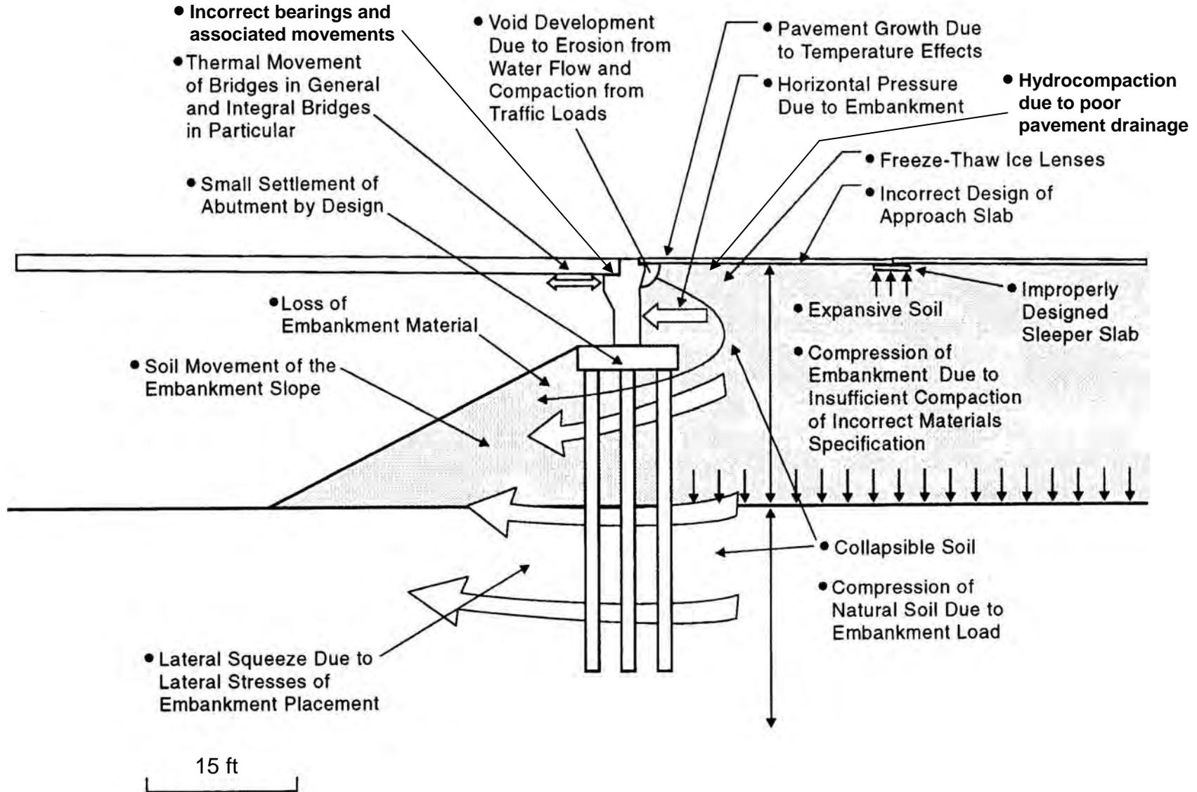
Figure 1-3. Problems leading to the existence of a bump (modified after NCHRP, 1997).
