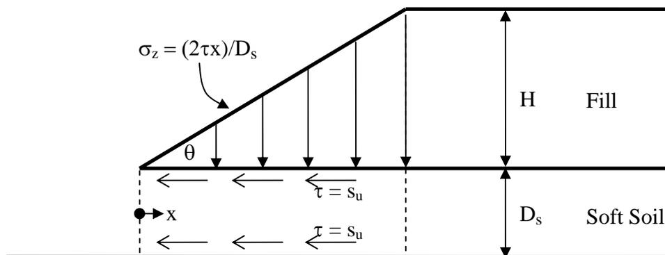
**Figure 1-20. Definitions for calculating safety factor against lateral squeeze (after Silvestri, 1983).**
