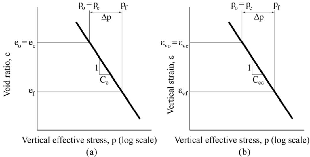
**Figure 1-10. Typical consolidation curve for normally consolidated soil, (a) Void ratio versus vertical effective stress and (b) Vertical strain versus vertical effective stress.**
