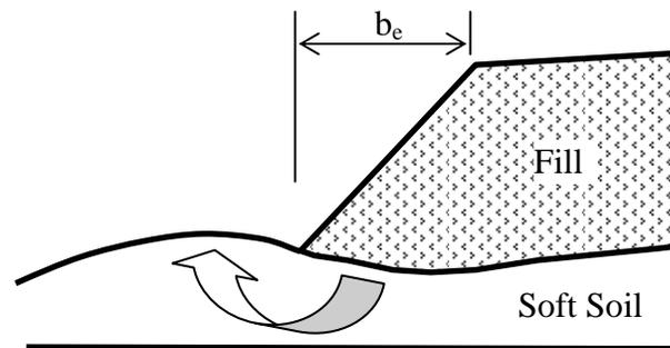
**Figure 1-18. Schematic of lateral squeeze phenomenon.**
