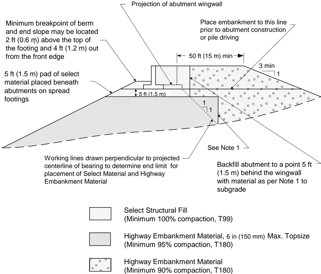
Note 1: Highway embankment material and select material shall be placed simultaneously of the vertical payment line
