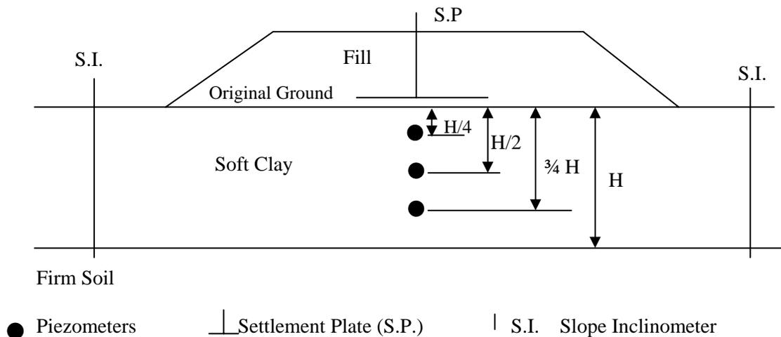
**Figure 1-23. Typical locations for various types of monitoring instruments for an embankment constructed over soft ground.**
