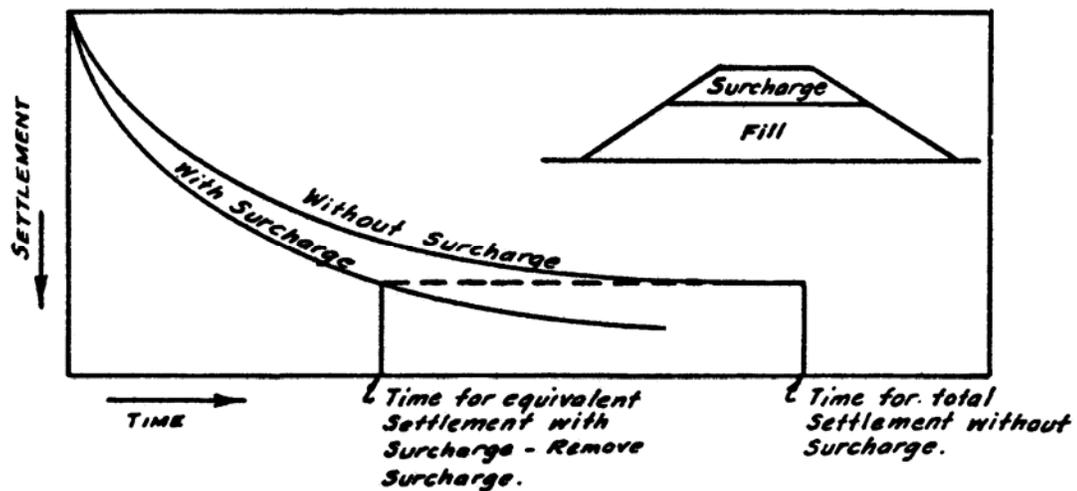
Figure 1-21. Determination of surcharge time required to achieve desired settlement.
