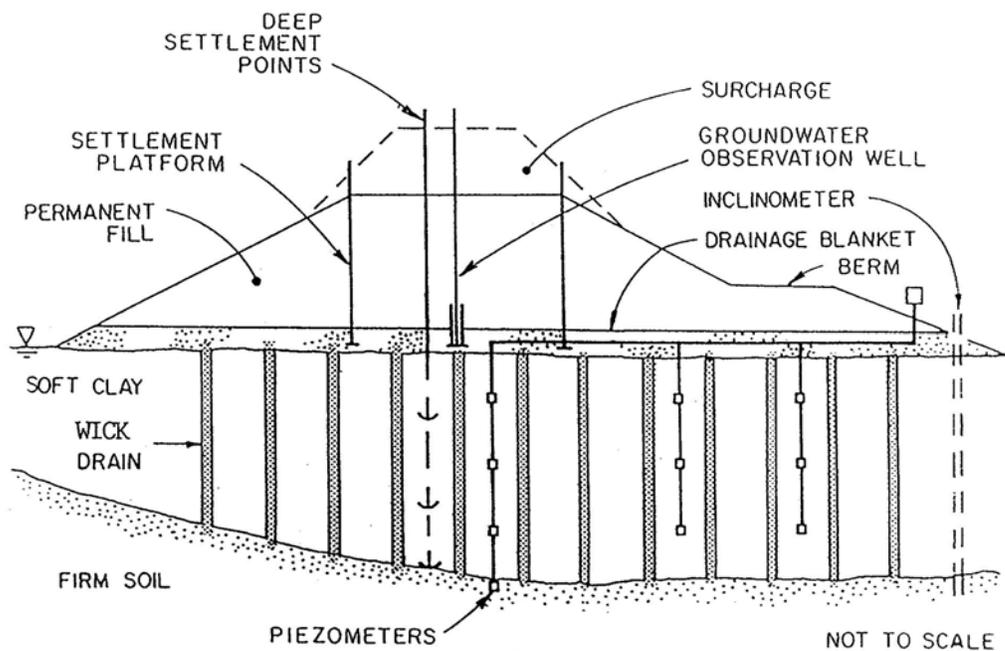
**Figure 1-22. Use of vertical drains to accelerate settlement (NCHRP, 1989).**
