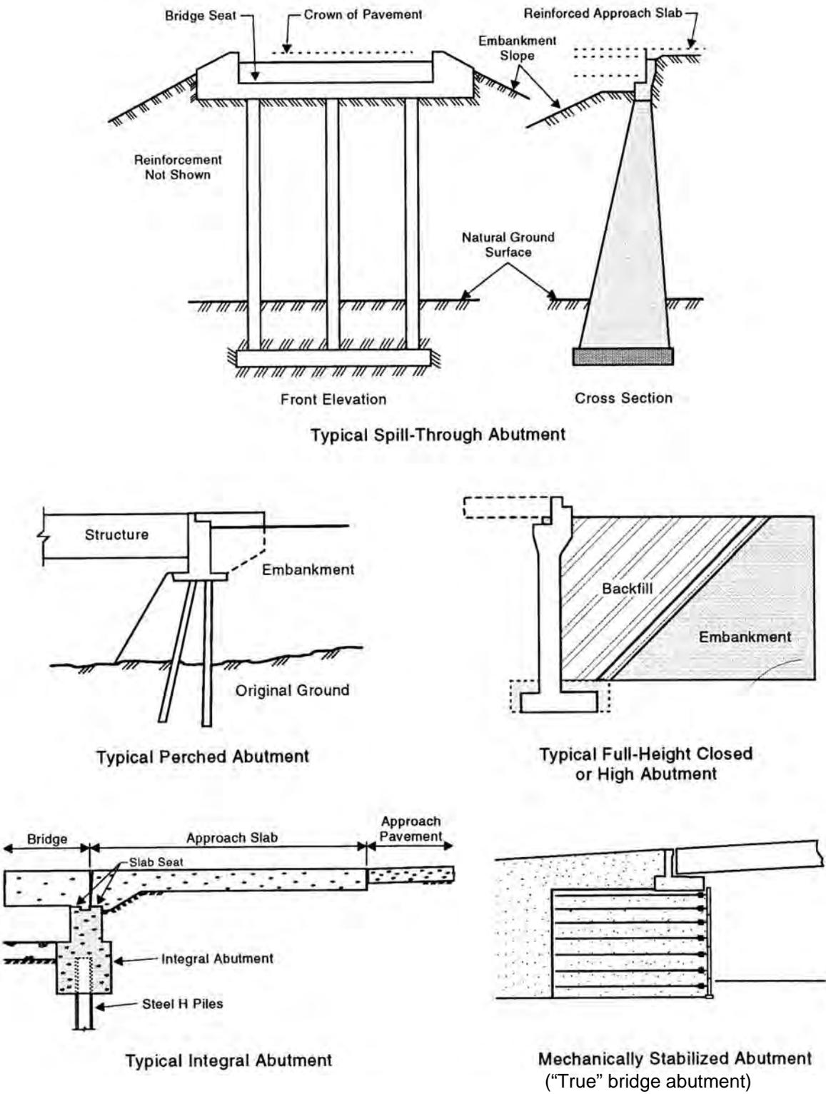
Figure 1-2. Types of abutments (modified after NCHRP, 1990).
