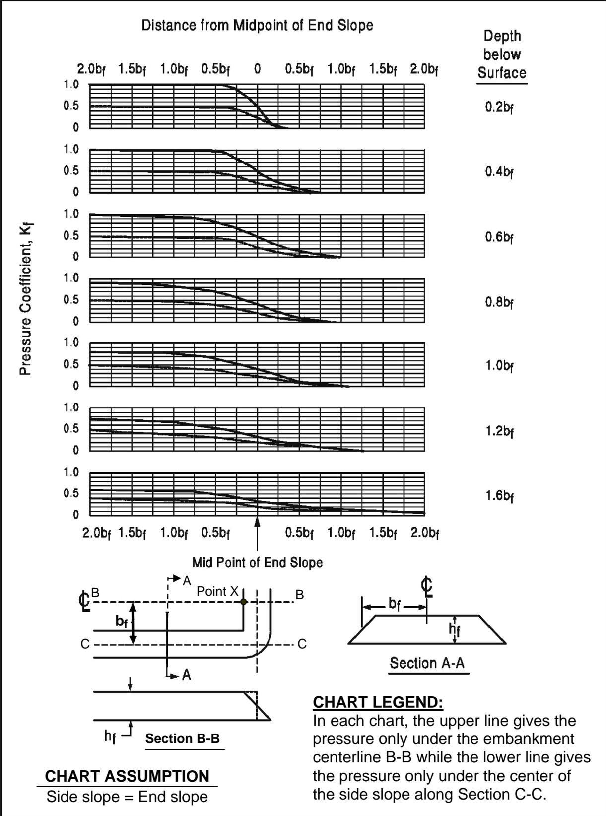
Figure 1-6. Pressure coefficients beneath the end of a fill (after NYSDOT).
