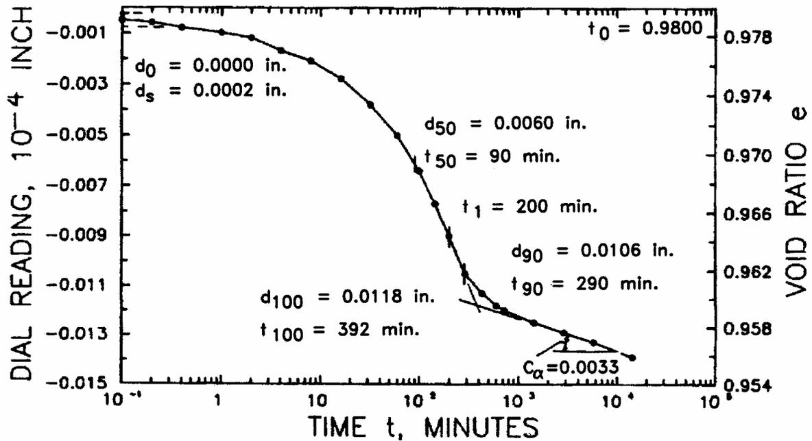
**Figure 1-17: Example time plot from one-dimensional consolidometer test for determination of secondary compression (USACE, 1994). (1 in = 25.4 mm)**
