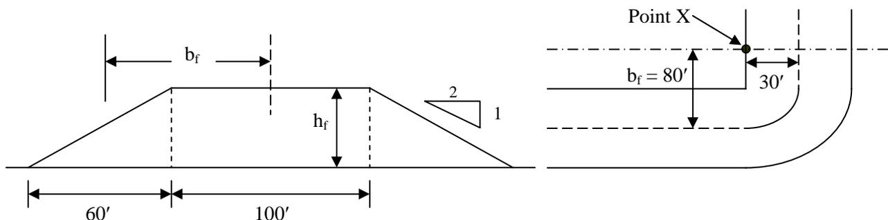
**Find:** The stress increase ( $\Delta p$ ) under the proposed abutment centroid (Point X) at a depth of  $0.8 b_f$  below the base of the fill.
