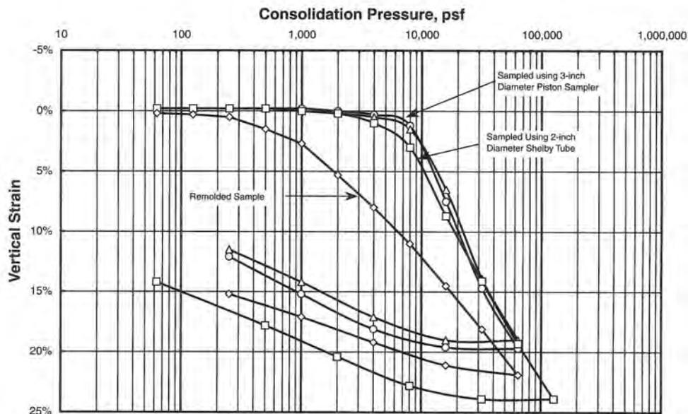
**Figure 1-8. Effect of sample disturbance on the shape of the one-dimensional consolidation curve (Reese, *et al.*, 2006).**
