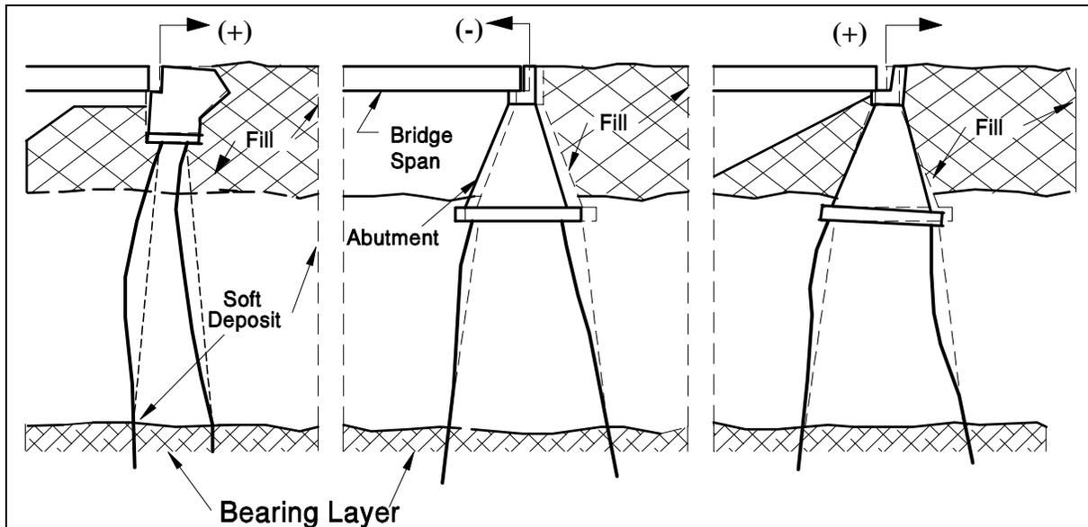
Figure 1-19. Examples of abutment tilting due to lateral squeeze (FHWA, 2006a).
