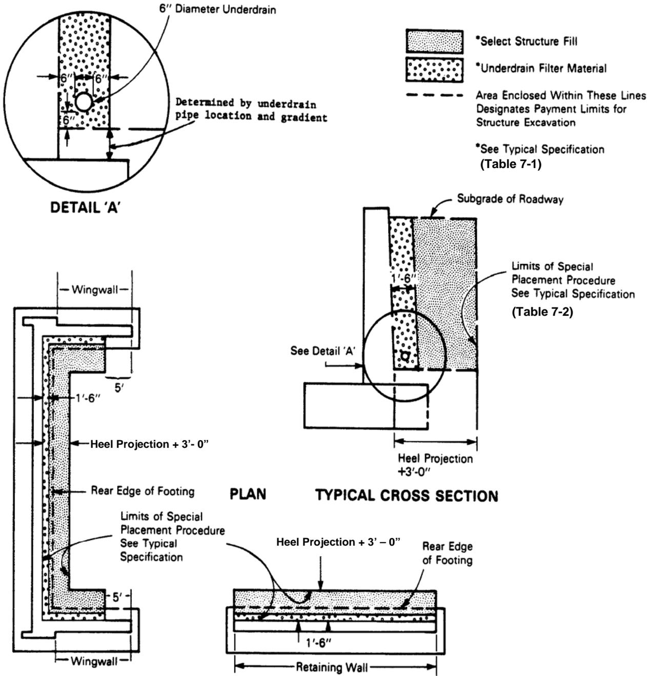
Figure 1-5. Structural backfill placement limits for porous drainage aggregate. (1 ft = 0.3 m; 1 in = 25.4 mm)
